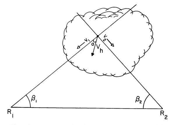
Figure 7. Measuring two-dimensional horizontal particle velocities by use of two Doppler radars observing the same storm from different directions.
