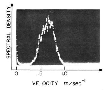
Figure 1. Doppler spectrum obtained in snow with a vertically pointing Doppler radar beam. Note the excellent velocity resolution of the system.
