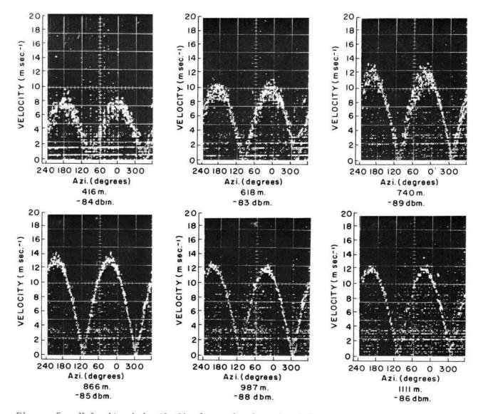
Figure 5. Velocity-Azimuth displays showing the CAR radial velocity at several altitudes. Radar beam elevation angle 20°. Radar site, Norman, Okla. Time 2023 to 2031 CST, 26 June. Signal mean intensity is indicated in -dbm.
