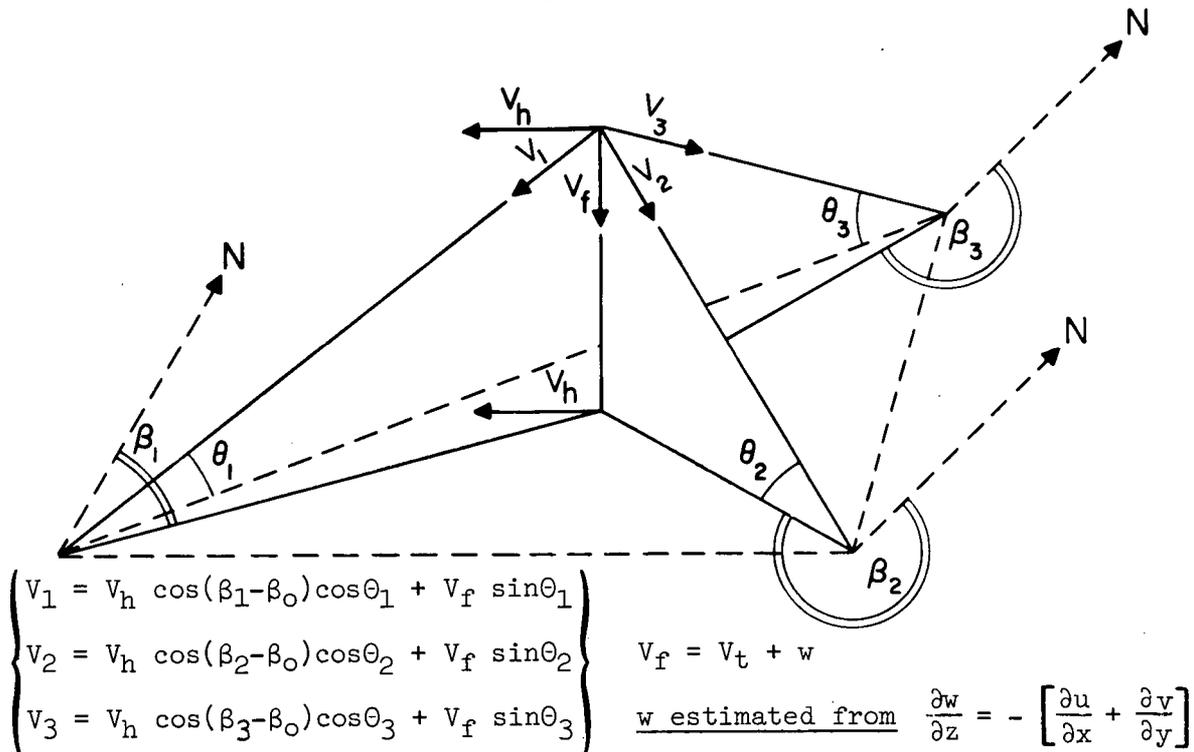
Figure 8. The three-Doppler radar method
