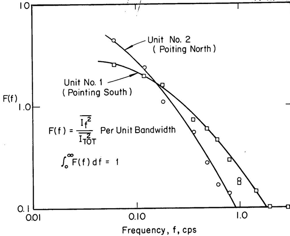
Figure 2. Spectra of light fluctuations.
