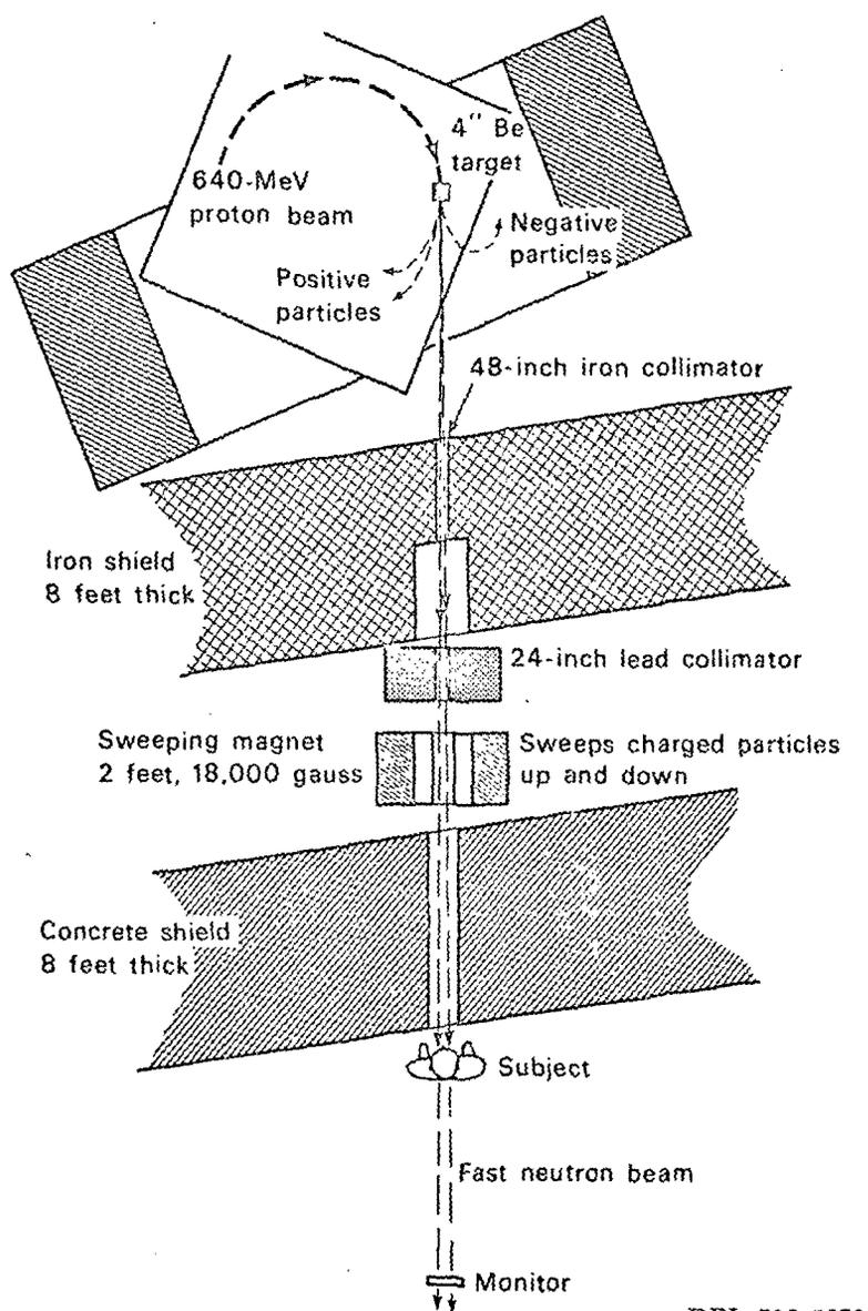
Figure 1a. Schematic layout of the Berkeley 184" cyclotron as it was used for observing light flashes from high energy neutrons (0.64 BeV maximum energy).
