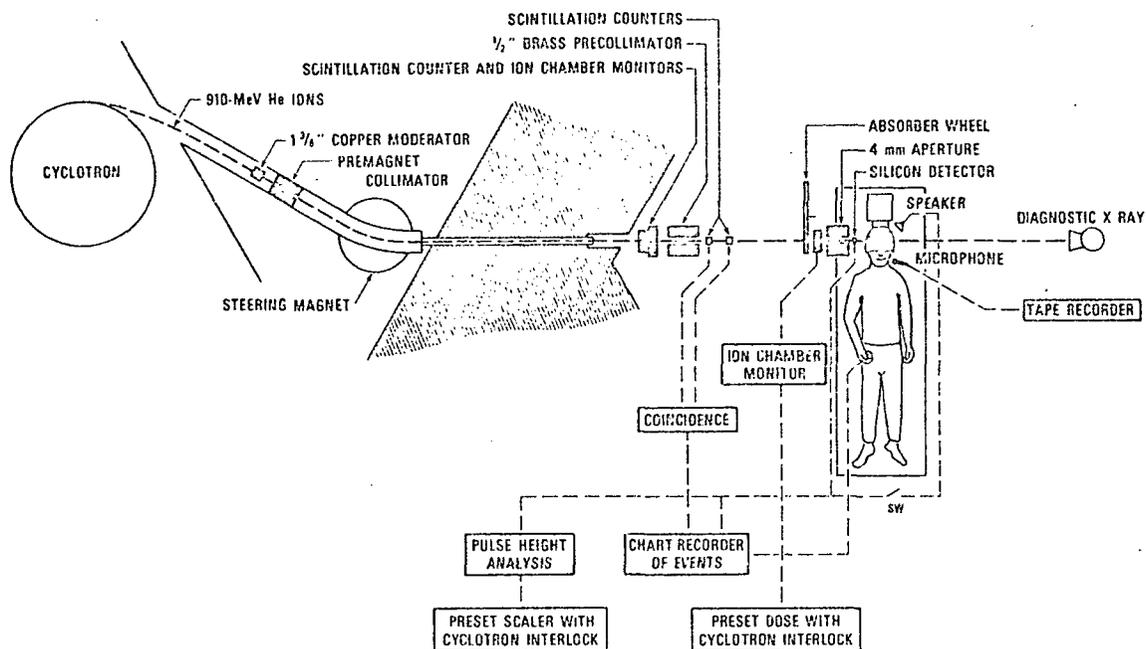
Figure 3. Schematic layout of the manner in which individual accelerated helium ions were passed through the left eye of dark adapted observers. The 900 MeV helium ion beam was moderated by absorbers to about 250 MeV kinetic energy, re-collimated and magnetically deflected. Each particle was individually monitored by means of a coincidence arrangement and a silicon detector.
