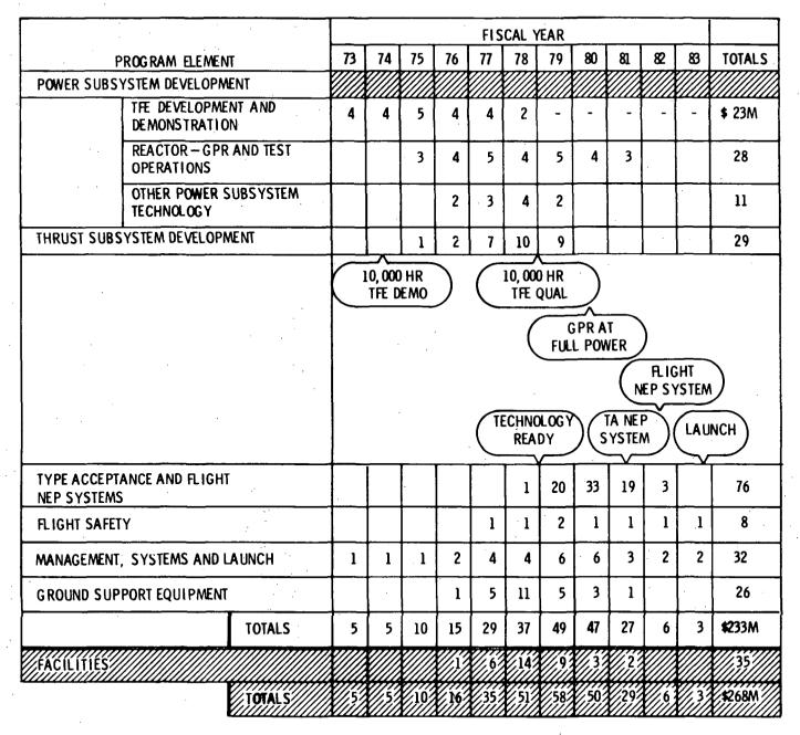
Key programmatic options and schedule milestones are compared for the NEP System development program alternates investigated. These alternates employ an extensive TFE development program and a Ground Prototype (flight configured) reactor test. In addition, the Baseline includes an earlier TREX reactor, which is not necessarily flight configured.
