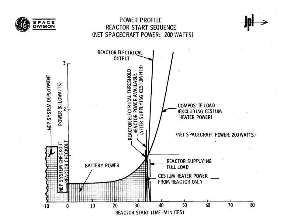
For a spacecraft with an arbitrarily assumed 1,000-watt net power requirement, the start-up batteries no longer are required 36 minutes after initiation of reactor start.
