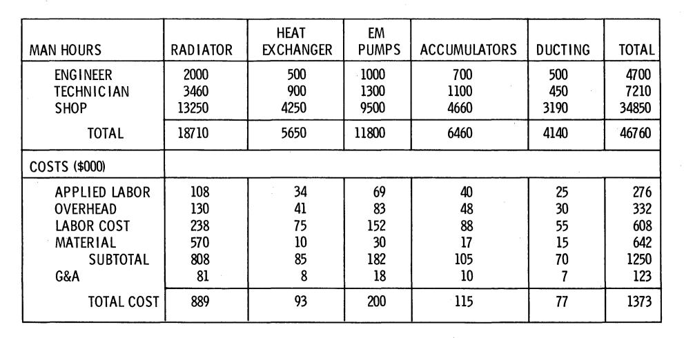
A detailed comparison of the cost for the main heat rejection radiator is shown, which is typical of the results for the other components.
