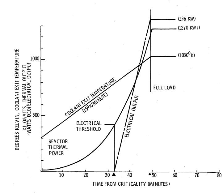
As the reactor thermal power level is increased during reactor start-up, the coolant flow is increased proportionally, maintaining a constant temperature differential across the reactor.
