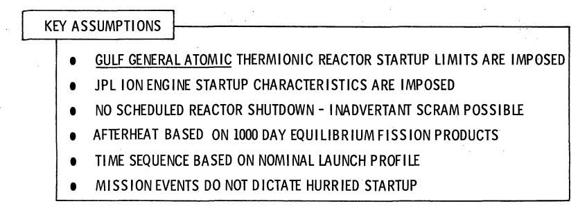
No electrical power is available from the reactor for use in the spacecraft until reactor start-up is completed (Step 4), a nominal two hours and 13 minutes after lift-off. Electrical power required during the time prior to Step 4 will have to be provided from other sources.
