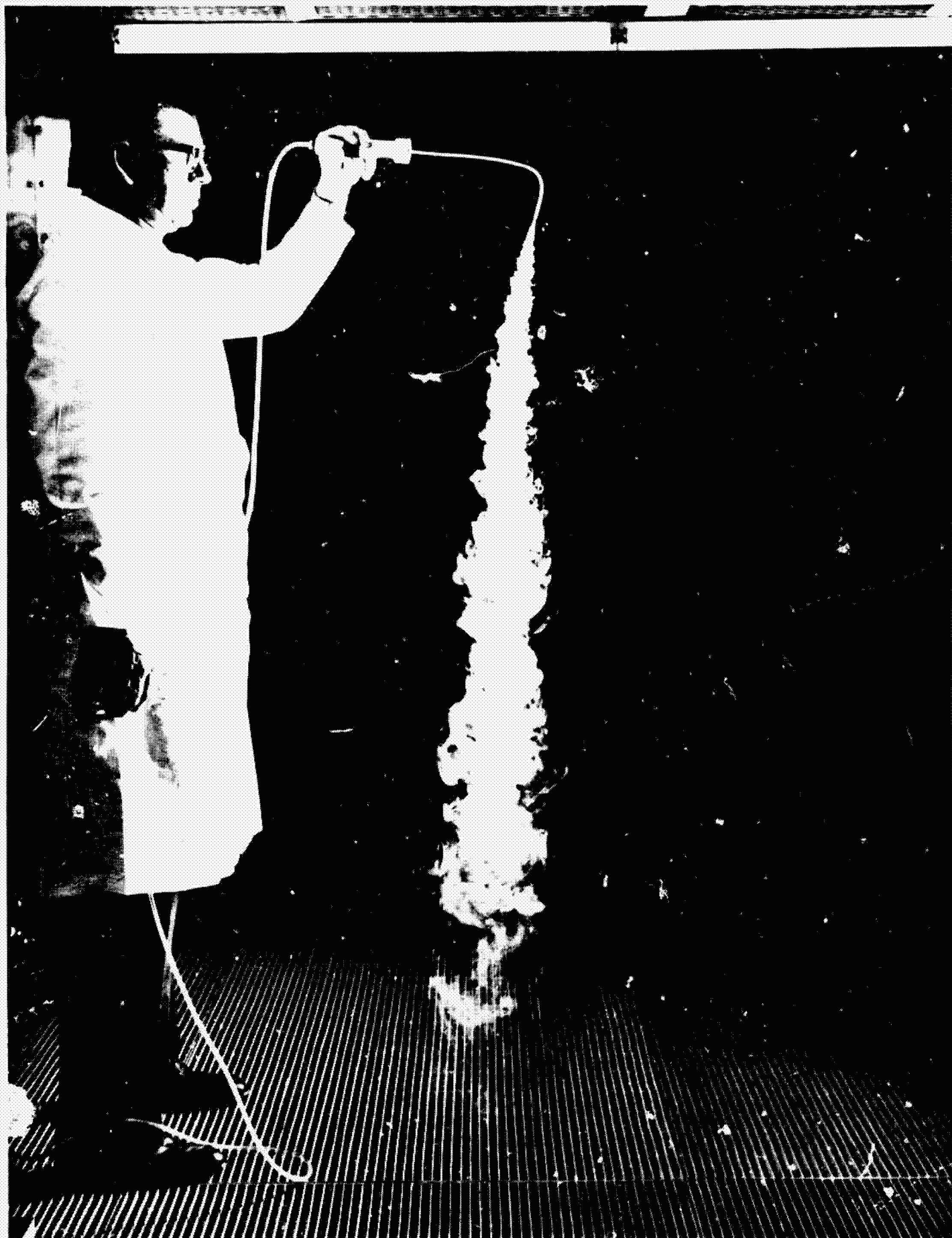
Figure 16 - Smoke Test in Vertical Laminar Flow Room
