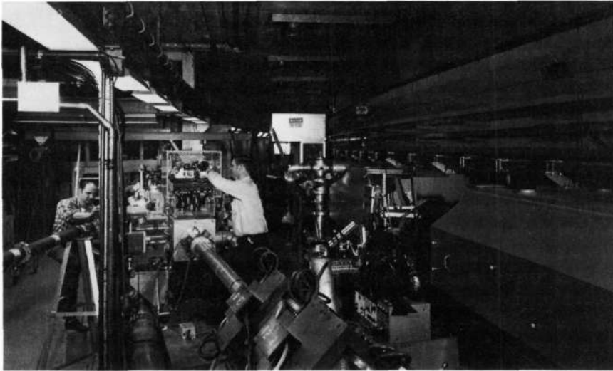
FIGURE 4.10 The AGS magnet ring and linac junction. This 33-GeV accelerator at the Brookhaven National Laboratory is the principal source in the United States for research using protons in the energy range 12 to 33 GeV. The AGS has been undergoing a major conversion that is now nearing completion. The purpose of this conversion is to provide higher-intensity beams of protons and secondary particles and increased experimental capability, thereby making it possible to carry out research of a qualitatively different character than before. [Source: Brookhaven National Laboratory.]
