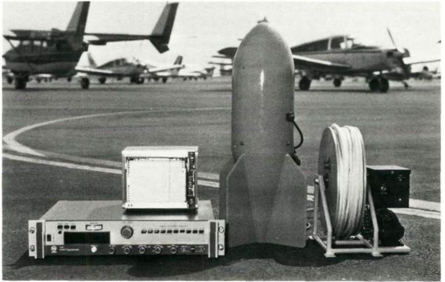
FIGURE 4.102 Photograph of a modern airborne proton magnetometer used for making magnetic surveys, which are particularly useful to petroleum geologists in helping to identify formations in which oil might be found. [Photograph courtesy of Varian Associates.]
