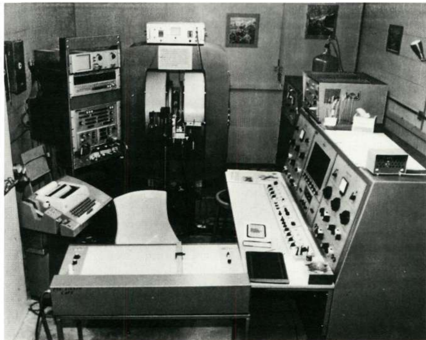
FIGURE 4.88 Bruker HFX-90 Multinuclear cw and pulsed FT NMR spectrometer consisting of (left to right) a Nicolet 1083 computer, magnet, and transmitter-receiver console. Variable-temperature and double-resonance capabilities are also present. [Photograph courtesy of the Department of Chemistry, Florida State University.]
