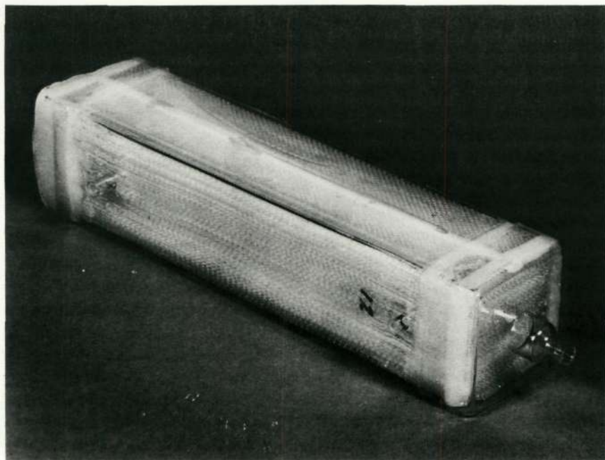
FIGURE 4.15 A preliminary version of a small, inexpensive ($15) artificial kidney, which has been developed at the High Energy Facilities Division of Argonne National Laboratory. It has been used successfully by nine patients at an Illinois Veterans Hospital. It has small enough volume ( 6 \times 2 \times 2 in. 3 ) to be suitable for a child, and it is hoped that it can be made inexpensive enough to be used daily. The basic configurations of these dialyzer designs are also being explored for their potential as membrane oxygenators for heart-lung machines. [Source: Argonne National Laboratory.]
