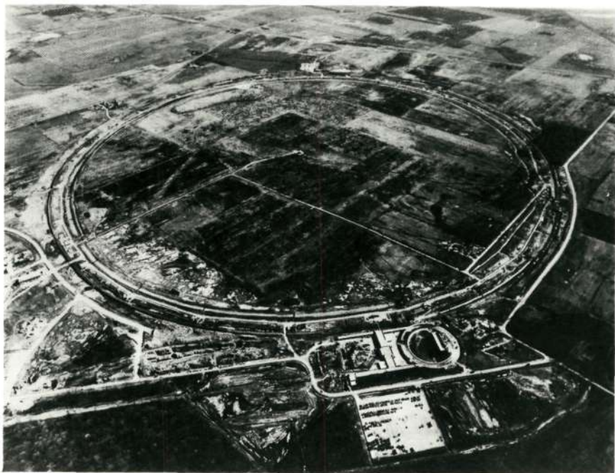
FIGURE 4.16 Aerial view of main accelerator at the National Accelerator Laboratory. This 200–500-GeV proton accelerator will be for some years the only controlled source of protons in the world for research in the energy range above 80 GeV and the only one in the United States above 33 GeV. In addition to proton beams, the accelerator will provide many beams of secondary particles—neutrinos, pions, kaons, photons, and antiprotons. [Source: National Accelerator Laboratory.]
