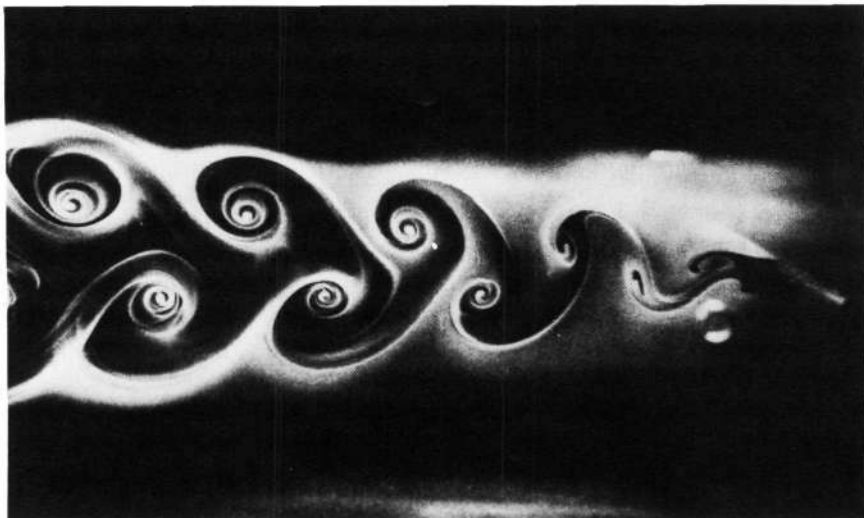
FIGURE 4.67 Air flowing past a cylinder rolls up into a regular succession of vortices. A cross section of these vortices is made visible by injecting a sheet of smoke in the center of a wind tunnel. (Photograph taken by Gary Koopmann at the Naval Research Laboratory, Washington, D.C.) [Source: Yearbook of Science and Technology 1971 . Copyright © 1971, by McGraw-Hill Book Company, Inc. Used with permission of McGraw-Hill Book Company.]
