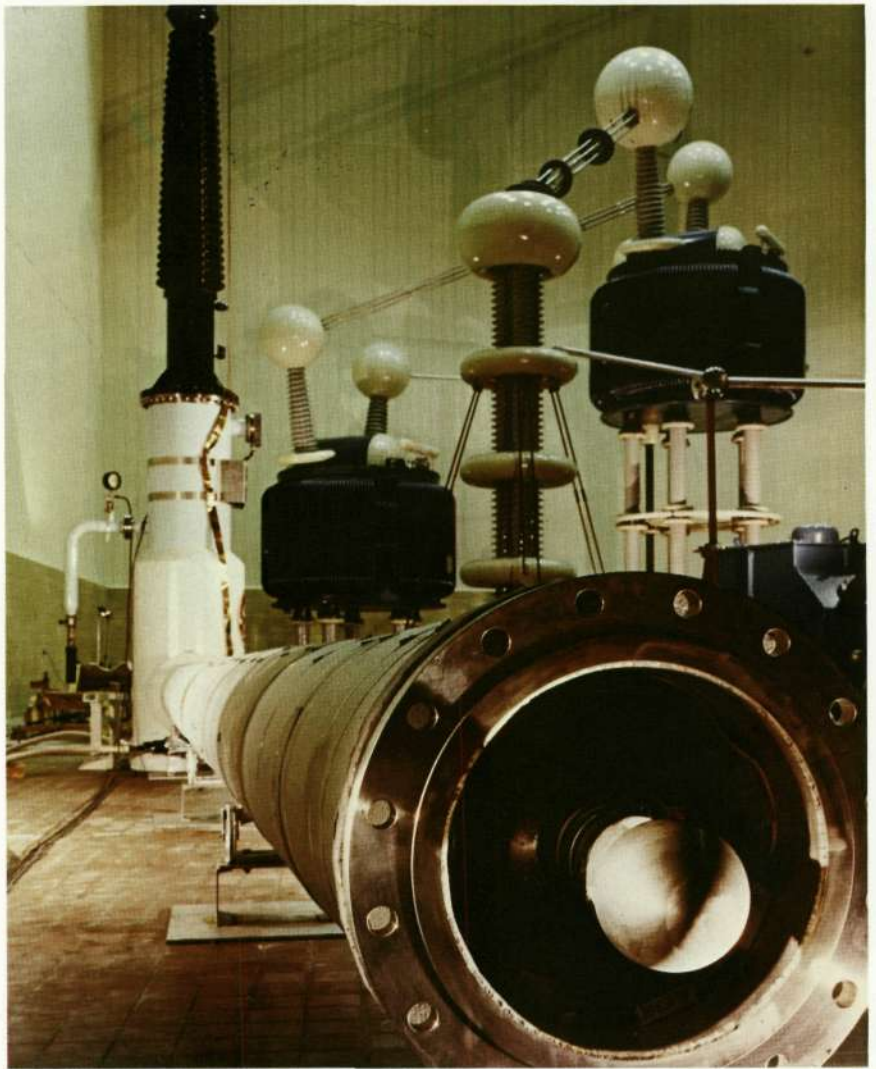
PLATE 4.IX A 40-ft section of high-voltage (450,000 V) cryogenic transmission cable undergoing testing at the General Electric Company.
