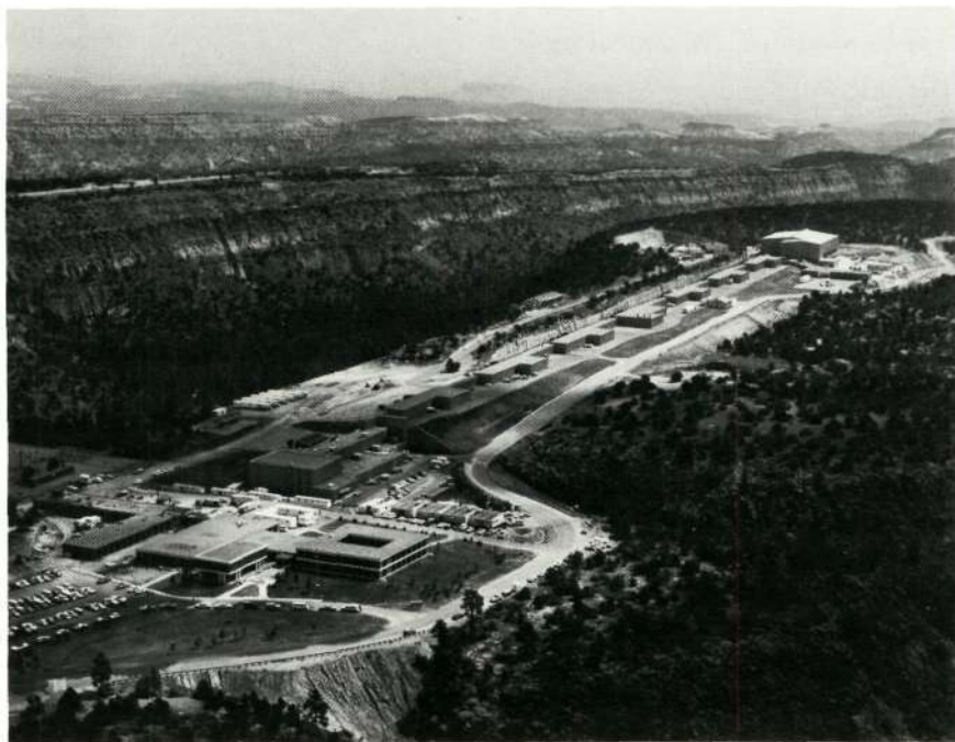
FIGURE 4.25 Aerial view of the Los Alamos Meson Physics Facility. This facility features 1-mA proton beam at 800 MeV, plus simultaneously either 100- \mu A hydrogen ions at 800 MeV or 1- \mu A polarized hydrogen ions at 800 MeV. Beams of protons, neutrons, muons, and neutrinos will be available for simultaneous use in a multidisciplinary program.
