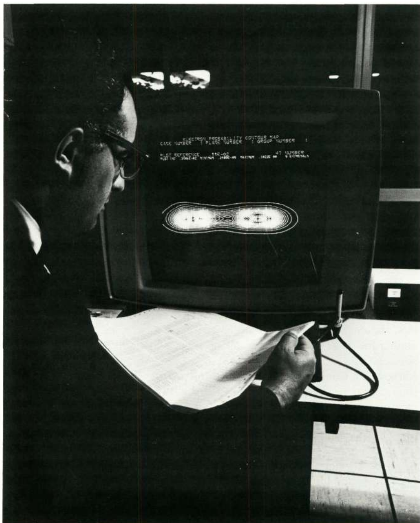
FIGURE 4.92 Computer-generated electron density map of the reaction \text{NH}_3 + \text{HCl} \rightarrow \text{NH}_4\text{Cl} , taken in a plane along the N-Cl axis, is projected on a display tube. [Courtesy J. D. Swalen, IBM Research Laboratory, San Jose, California.]
