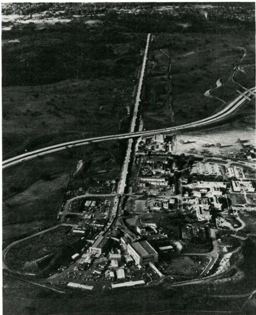
FIGURE 4.9 Aerial view of the Stanford Linear Accelerator Center. The 22-GeV electron accelerator at this center is the only controlled source of electrons in the world for research in the energy range above 12 GeV. In addition to electrons, this accelerator can provide many beams of secondary particles—pions, muons, kaons, and neutrinos. [Source: Stanford Linear Accelerator Center.]
