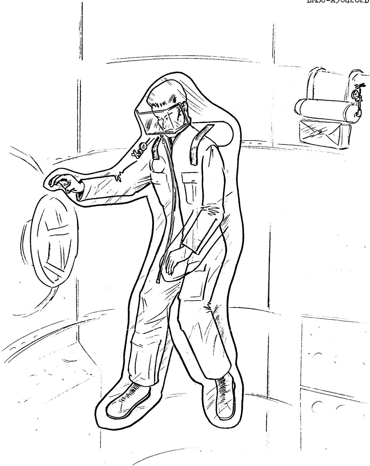
Fig. 11-3 Emergency Pressure Garment for Crewmen in Shirtsleeves
