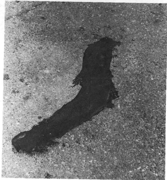
FIGURE 2a MIXING AND APPLYING EXPERIMENTAL QUANTITIES OF THERMOPLASTIC MATERIAL
