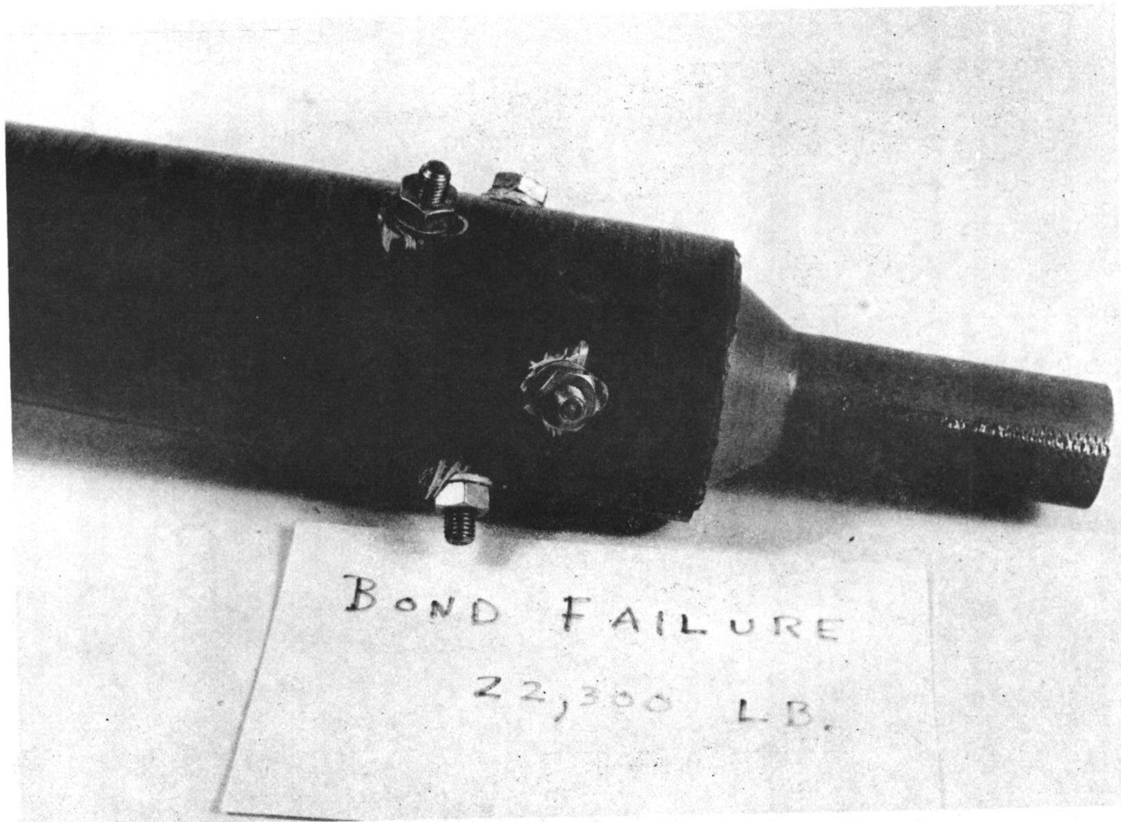
FIGURE 5-5. COMPRESSION END FITTING FAILURE IN BORON/EPOXY TUBE
