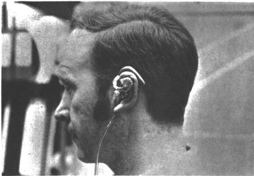
Figure 17. NASA ear oximeter.
