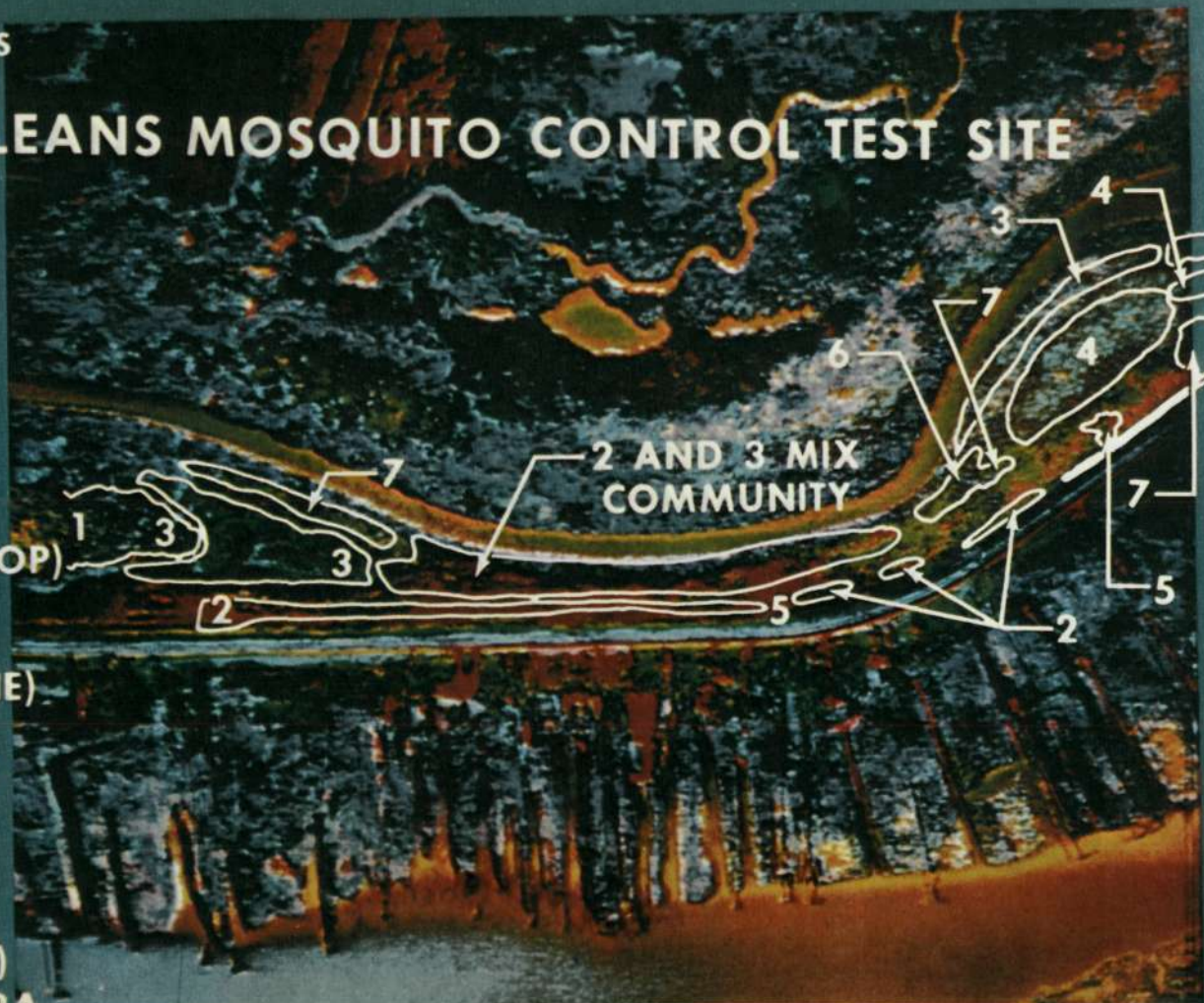
Figure 16.- This photograph acquired by the same means as the preceding three, was derived by adding the red and near infrared bands. This process enhances the ease of identifying the different vegetative communities and sharply delineates edge effects and community interfaces by assigning false colors to differentiate subtle density differences.
