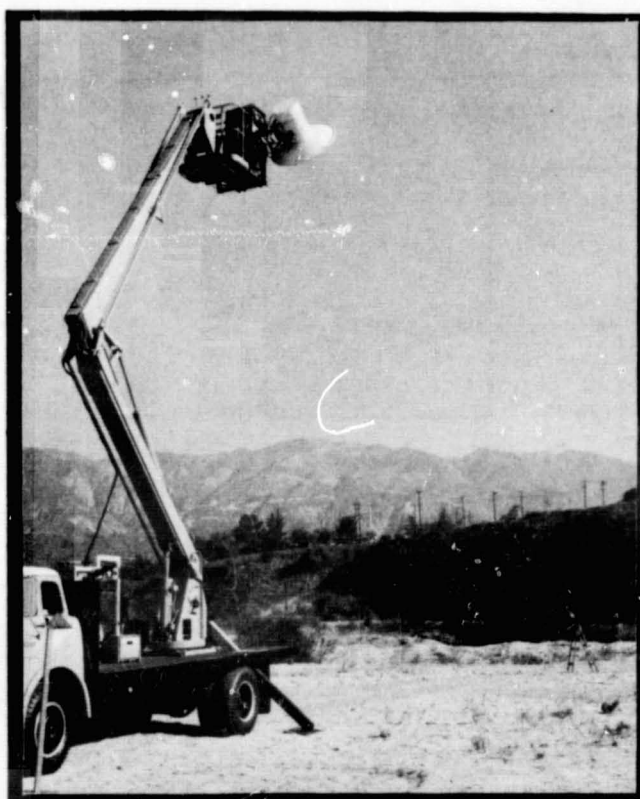
Figure 1. The radar radiometer is mounted on an aerial platform truck for access to areas of interest for remote sensing applications. The Luneberg lens and corner reflectors provide calibration targets for radar calibration.
