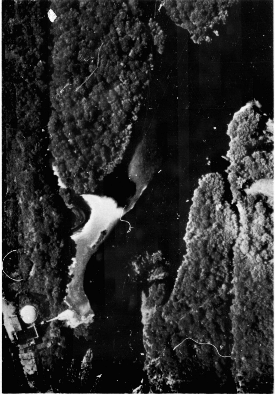
Figure 2.- IR Aerial photograph of paper mill waste entering Wisconsin River near Mosinee, Wisconsin.
