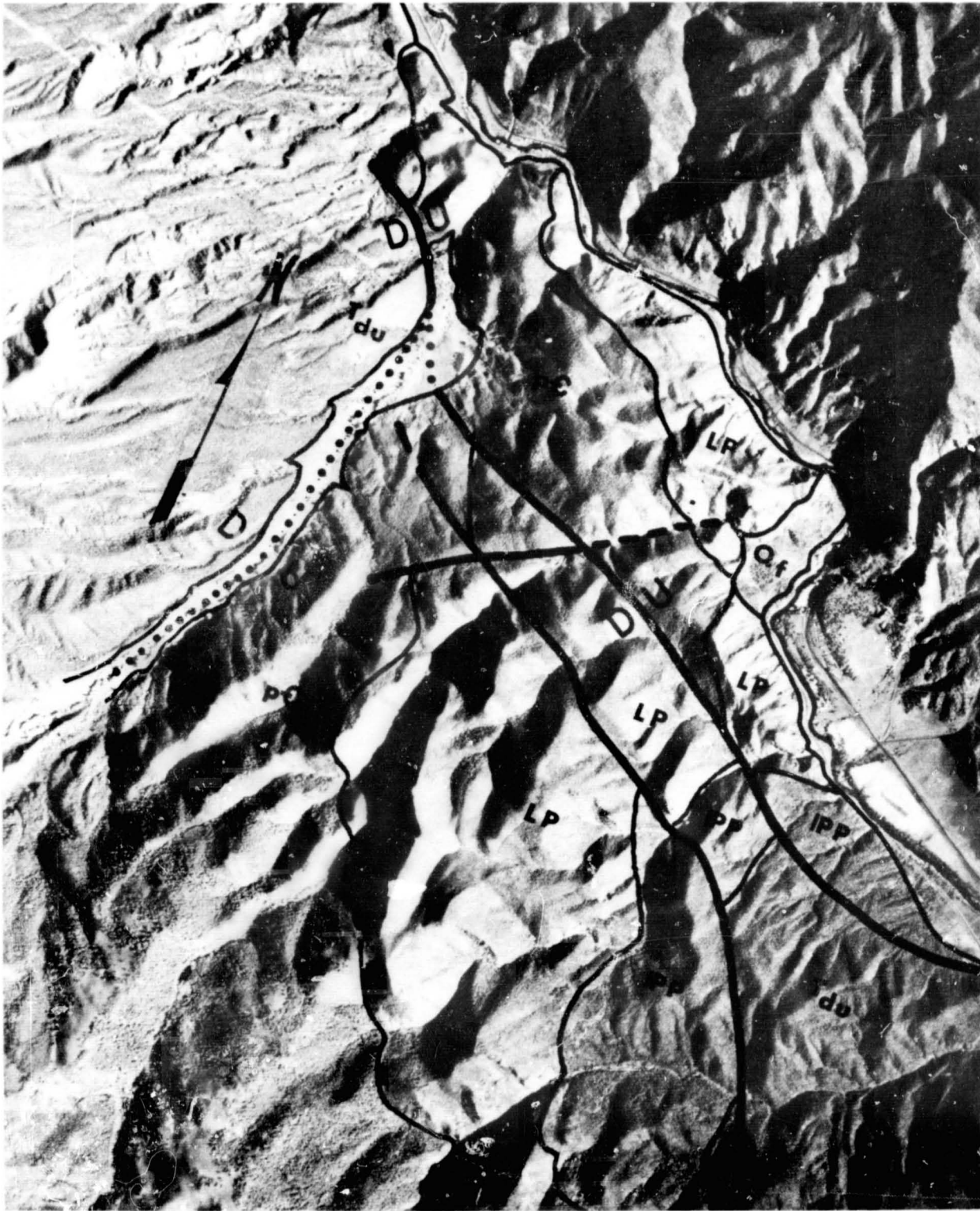
Figure 8.- Low sun-angle photograph near Salida, Colo. Type 2424 film with W25 filter. Sun angle 20^{\circ} . (pC, Precambrian; LP, lower Paleozoic sedimentary rocks; PP, Permo-Penn sedimentary rocks; Tdu, Dry Union Fm; Qf, fan.)
