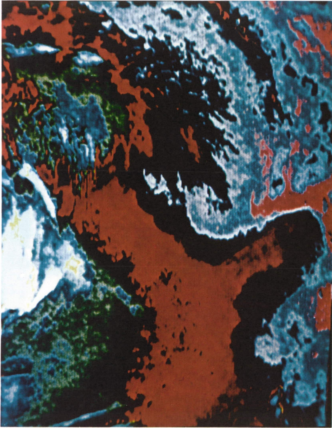
FIGURE 7. 32 level false color enhancement of ITOS HRIR Image of 27 Jan 71 showing warm Gulf Stream in red and light blue and cooler shelf waters in black.
