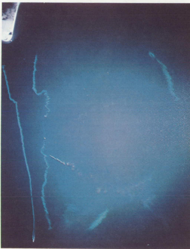
FIGURE 11. POINT AND LINE DYE SOURCES BETWEEN DRUM AND FISHING POINTS, 14 MAY 1971 (0848 EDT).
