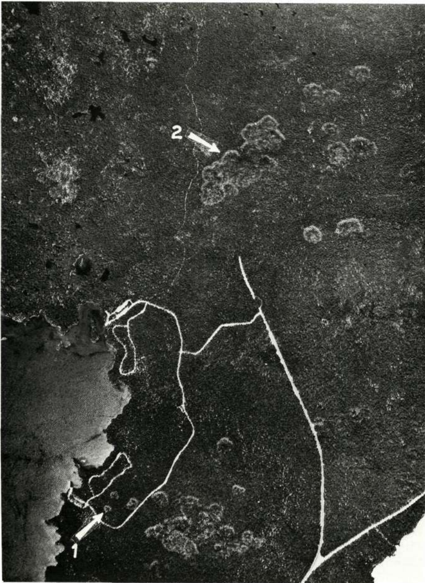
Figure 3.- 1:31,680 scale vertical of Waldo Lake test site showing Poria weirii root-rot signature in high Cascades of Oregon. Note "ringworm" pattern of bare ground openings caused by root-rot disease. Single patterns (1) range from 100 feet to 700 feet in diameter. Coalescing patterns (2) range up to 3,000 feet.
