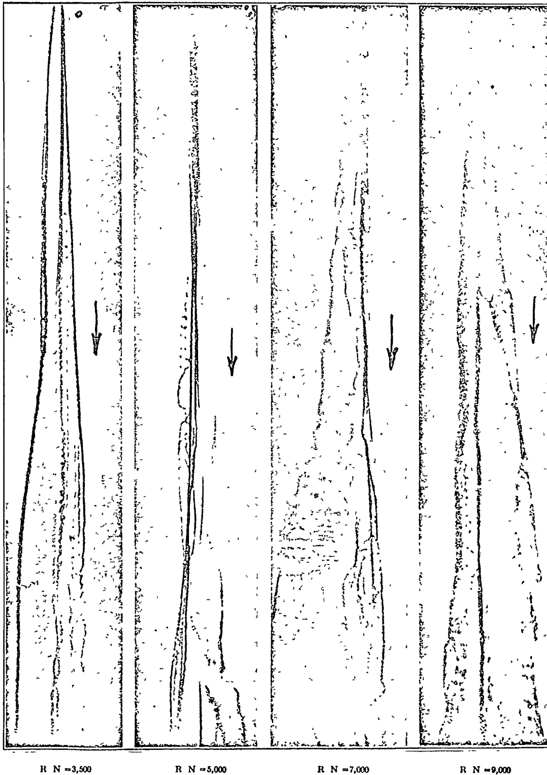
FIGURE 3—Fuel jets at various Reynolds Numbers, in vacuum, \times 25 Orifice diameter, 0.020 inch, air density, 0.0013 atmosphere (pressure = 1 mm Hg, absolute), fuel viscosity, 0.102 poise at 22^{\circ} \text{C} , photographs taken just beyond the orifice 3
