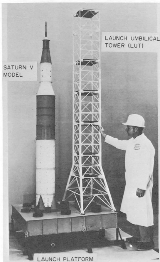
Figure 42.—One fortieth scale model of the Apollo-Saturn V space vehicle.
