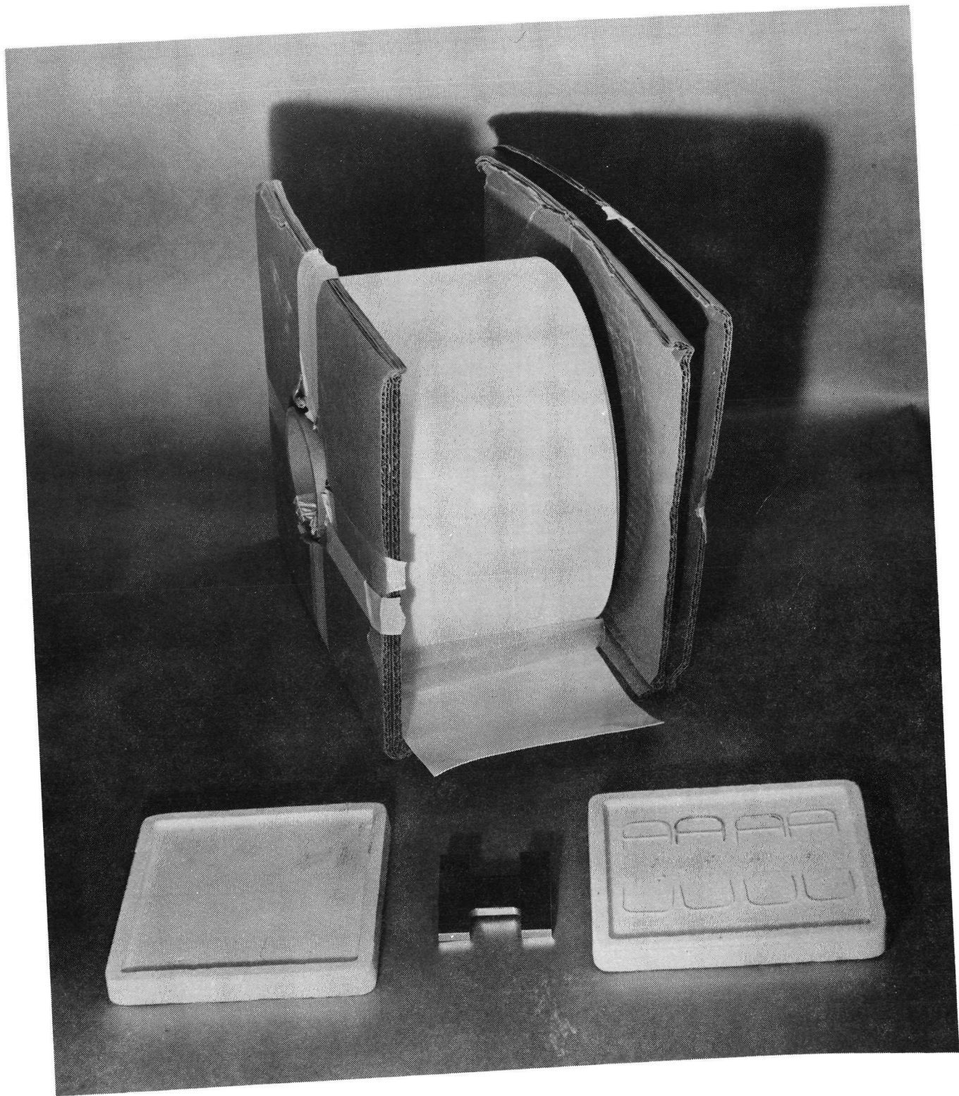
Fig. 65 A ROLL OF CERAMIC GREEN TAPE AND SAGGERS USED FOR SINTERING CERAMIC PARTS
