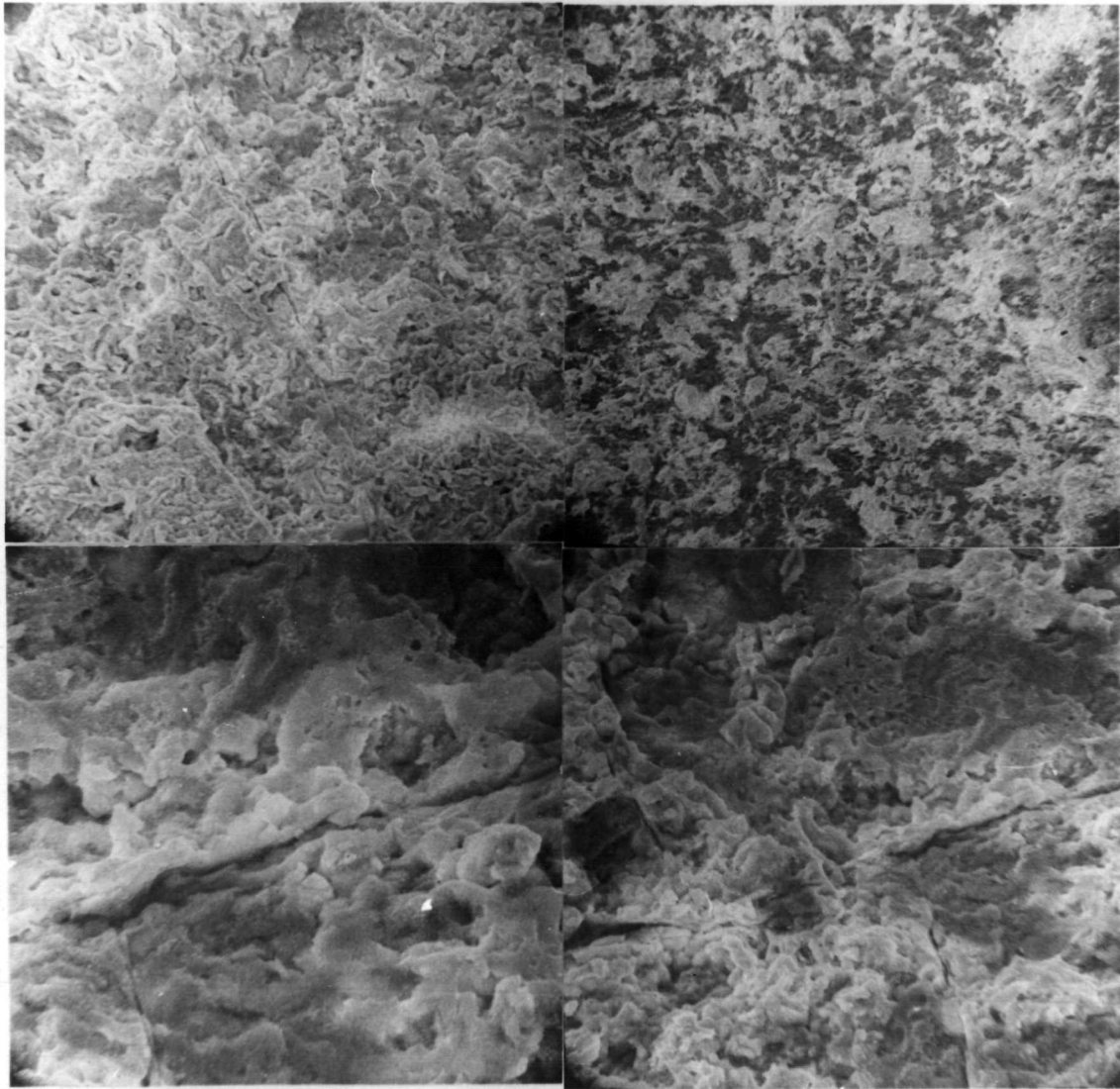
Plate 9 SEM micrographs of R512E, furnace cycled in air, 5 times to 2400° F. All same area. Upper right 200x, upper left 500x, lower right 1000x, lower left 2000x.
