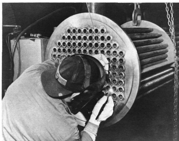
FIGURE 24.—Manual gas tungsten-arc welding of tube-to-header joints in Inconel 600.
