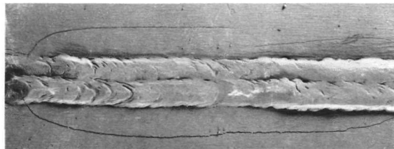
FIGURE 14.—Failure attributed to residual stress in 2-in.-thick Inconel X after aging at 1300° F for 20 hr. (The base metal was aged prior to welding.)
