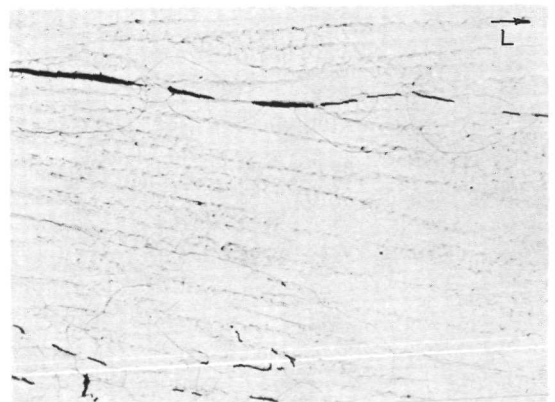
FIGURE 53.—Weld fissures in a nickel-chromium-iron alloy.
