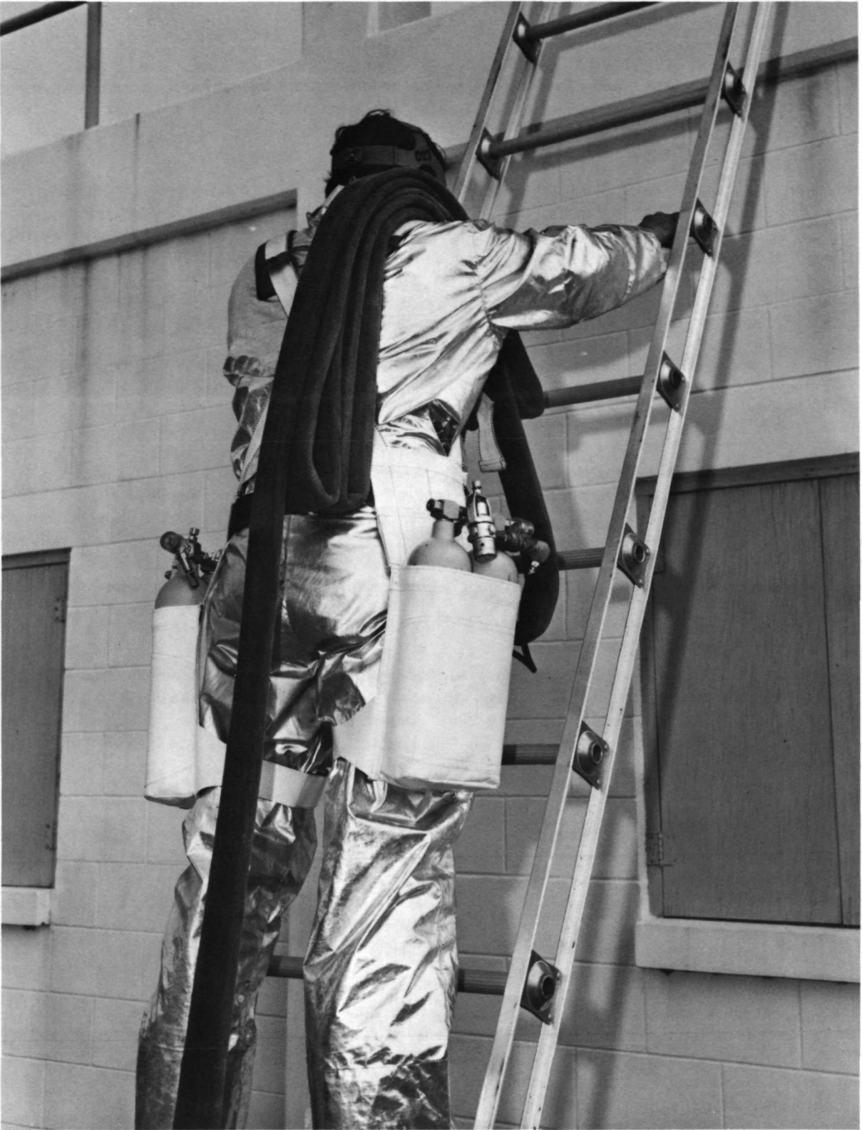
Breathing apparatus developed at Kennedy Space Center has superior human factor features incorporated in its design. Note pressure vessels mounted at the hips of the rescue team member.
