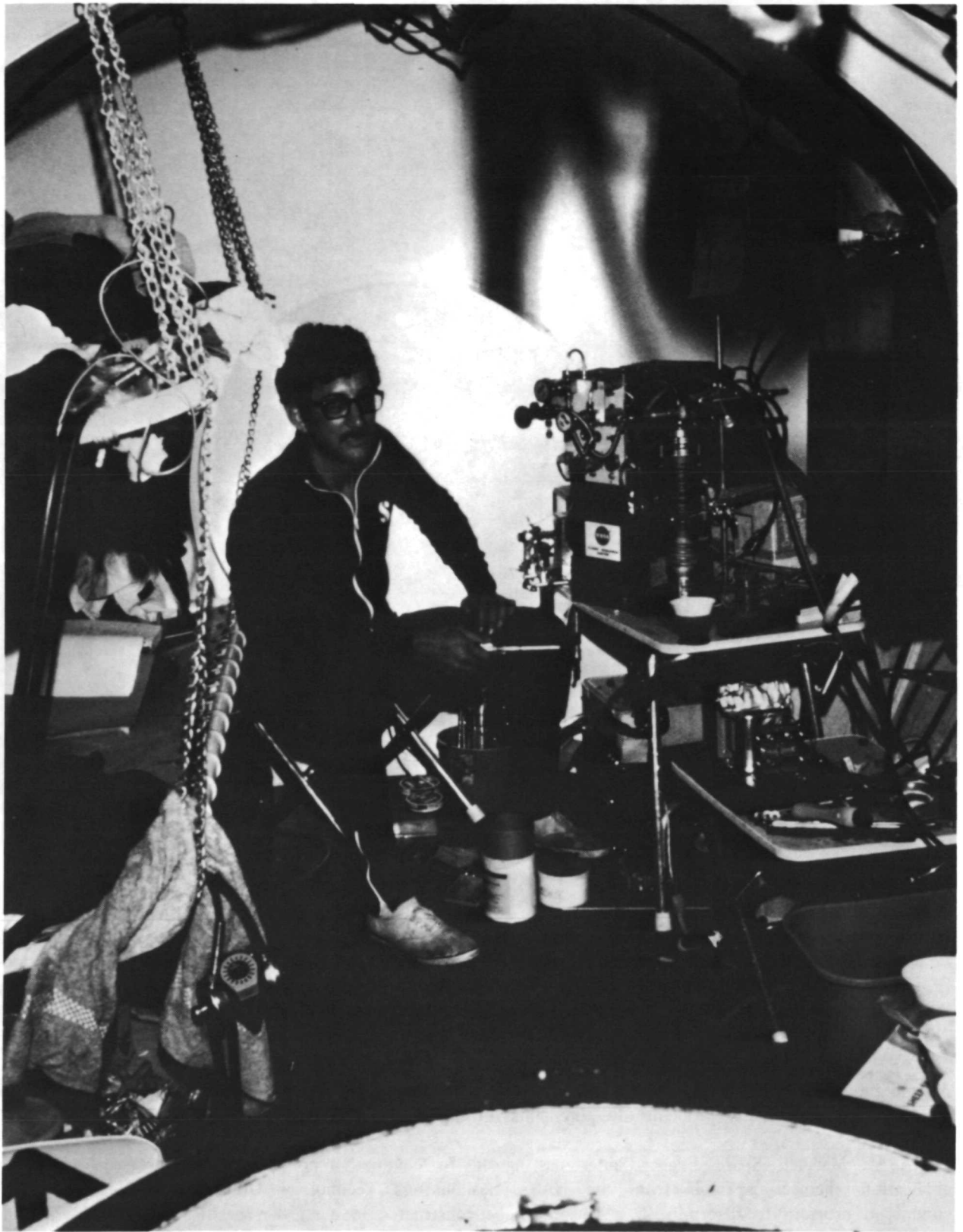
Researcher using mass spectrometer in Perry Hydro-Lab at a depth of 50 feet of sea water off the coast of Grand Bahamas.
