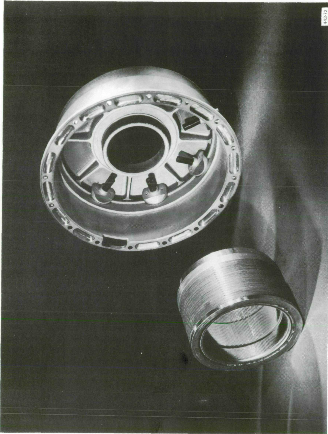
Figure 4-5 - Orbit Gear and Stator Housing (Flightweight)
