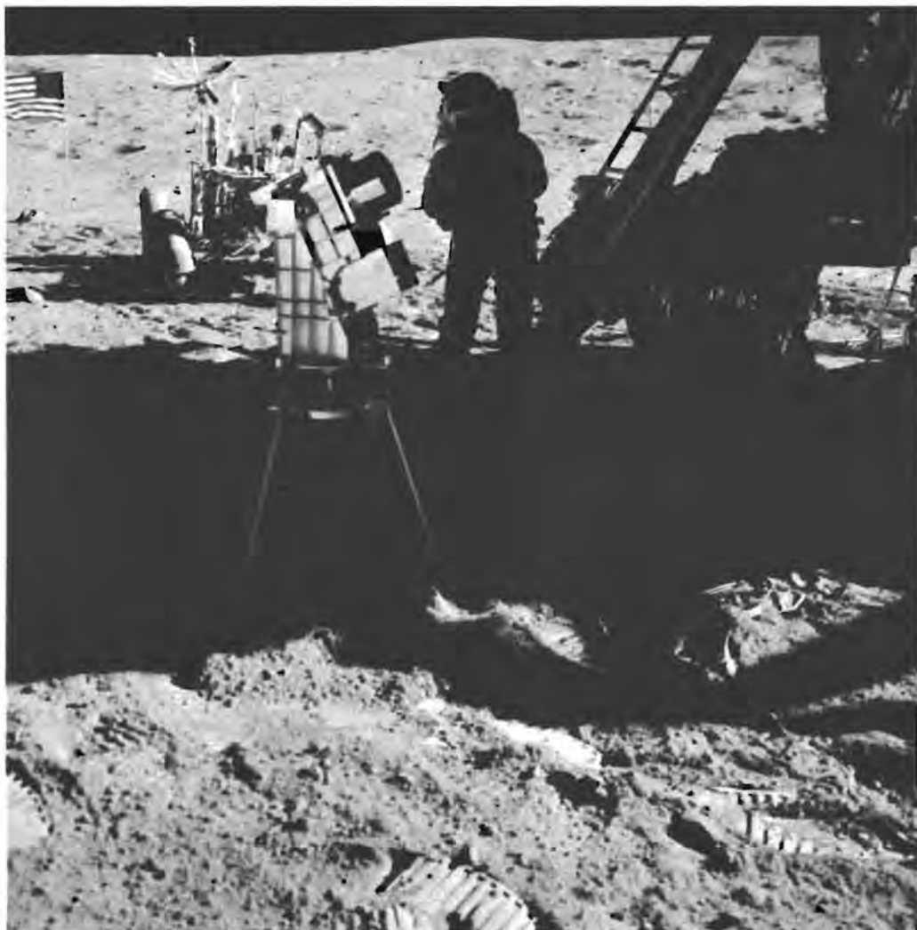
Figure 4-8.- Far ultraviolet camera/spectroscope experiment,
