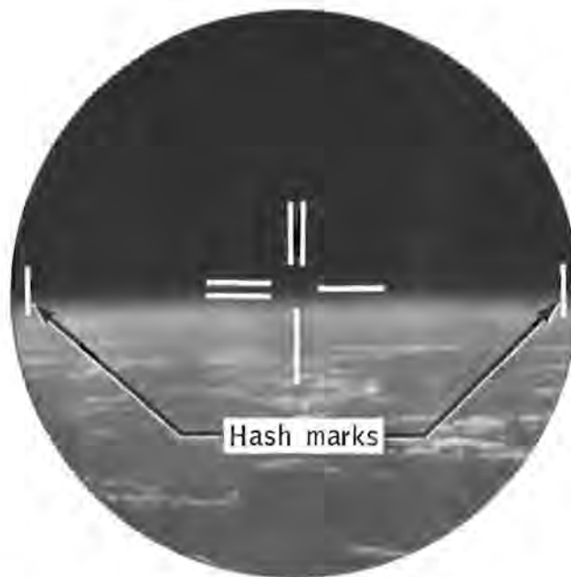
Figure 9-3.- Sighting through sextant for cislunar navigation training.
