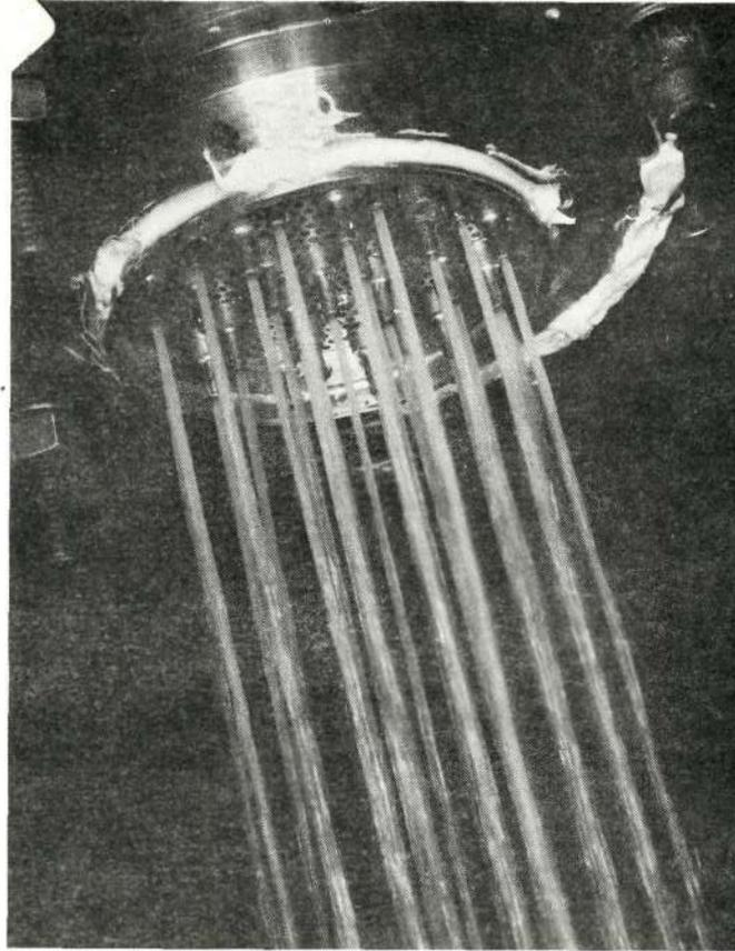
OXIDIZER CIRCUIT COLD FLOW SETUP
