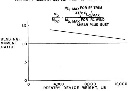
BENDING-MOMENT RATIO 250 SQ FT REENTRY DEVICE, MODIFIED TITAN LOT "J"
