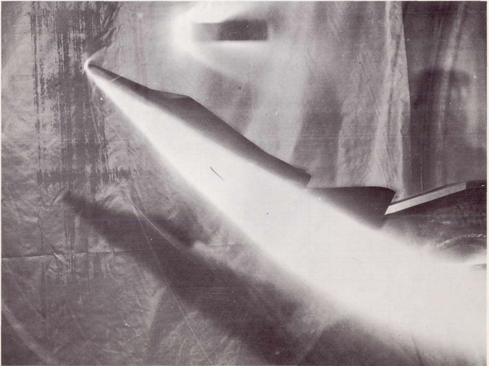
Figure 11.- White hot shock layer surrounding an X-20 model undergoing test.
