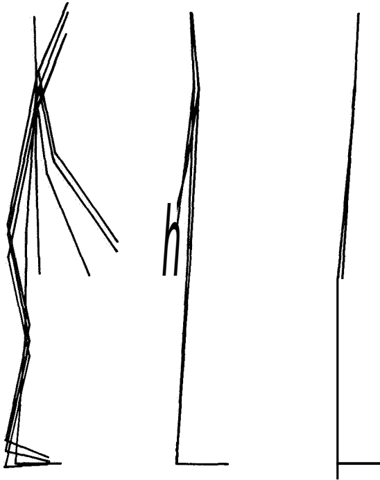
FIGURE 8.—Simulation results: free fall with subsequent stand erect.
