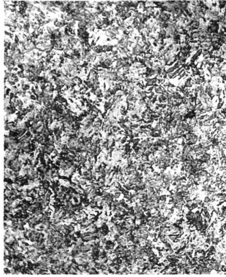
FIGURE 19A - MICROSTRUCTURE OF CUSTOM 455 STAINLESS STEEL ALLOY BAR AGED AT 1000°F (538°C) Etchant: HCl-Nitric Acid-Glycerine Mixture
