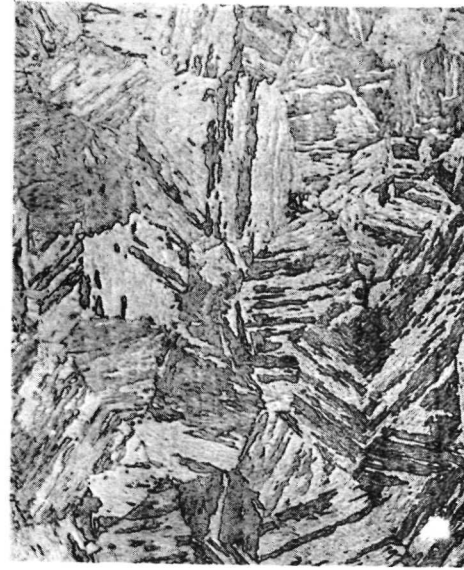
FIGURE 19B - MICROSTRUCTURE OF CUSTOM 455 STAINLESS STEEL ALLOY SHEET AGED AT 1000°F (538°C)
