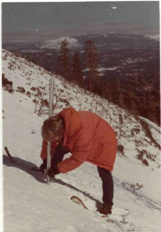
Figure 4.7. In addition to the 25 snow courses maintained by the California Cooperative Snow Survey in the Feather River Watershed, FRSL personnel have located a series of permanent snow survey field plots (white triangles, top photo) in the Bucks Lake Test Site in areas considered to be reasonably accessible during the winter months. During each suitable U-2 overflight, the field crew measures, using a Mount Rose snow sampling tube set, snow depth, snow condition and water content at each permanent plot.
