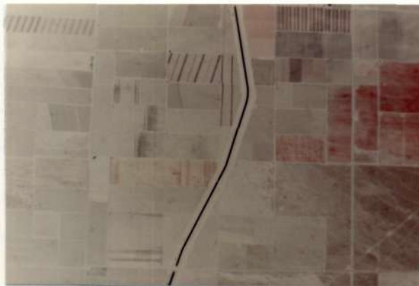
Figure 6.7. Line sprinklers and row-flooding east of Taft. The row-flooding techniques can be seen just west of the California Aqueduct in the center of the photo. The characteristic pattern of the latter technique is a dark return fading into lighter tones across a field, caused by the release of water at one end of the field which then spreads across the field.
