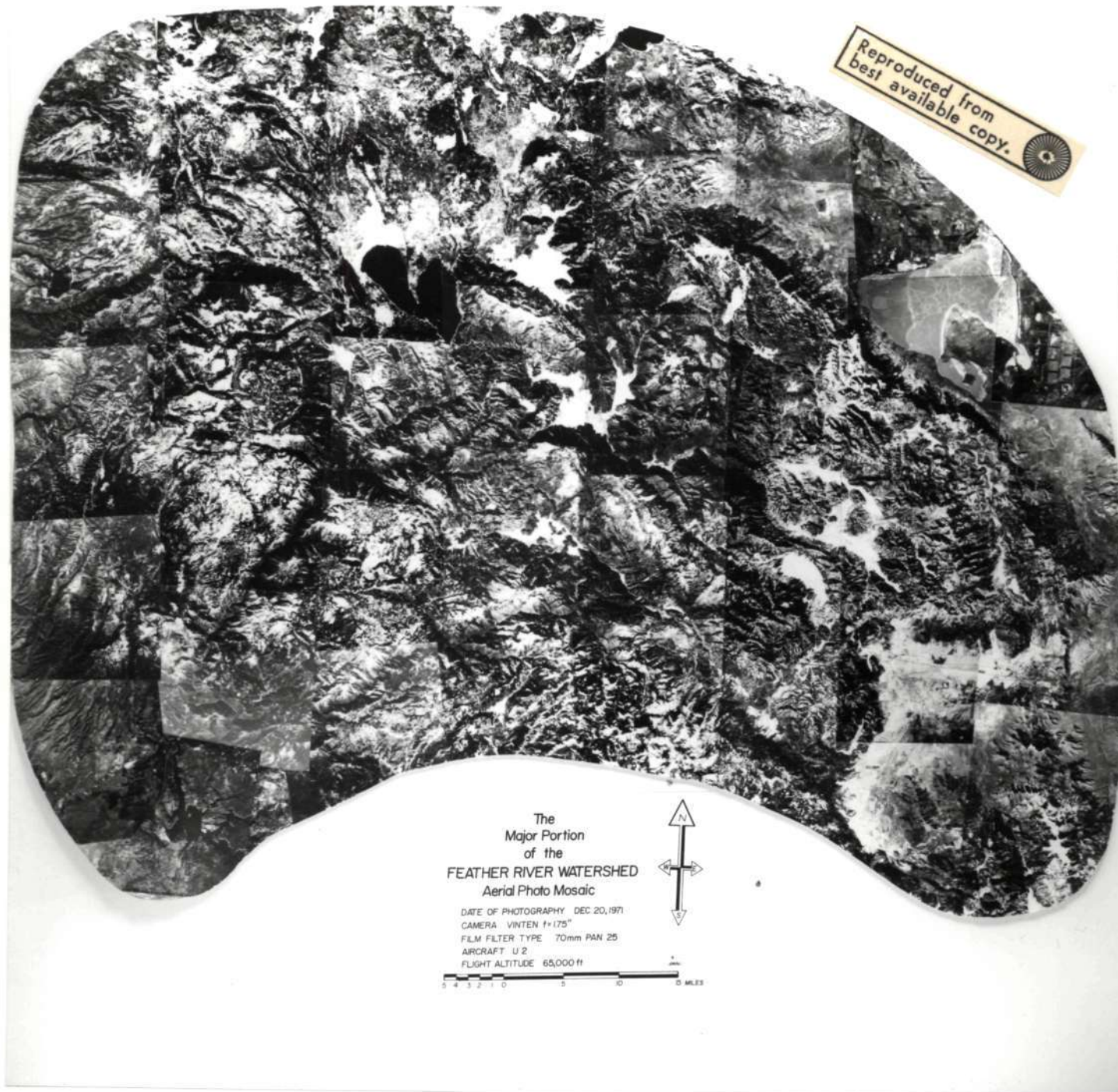
Figure 4.6. The U-2 imagery currently being procured on an 18-day cycle over the entire Feather River Watershed will be analyzed for determining the accuracy with which snowpack boundaries can be mapped. Coverage obtained on December 21, 1971 is shown here in the form of an uncontrolled photo mosaic. FRSL field crews have established additional snow survey ground plots within the Bucks Lake test site. These sites are visited each time suitable U-2 high flight imagery is acquired over the area.
