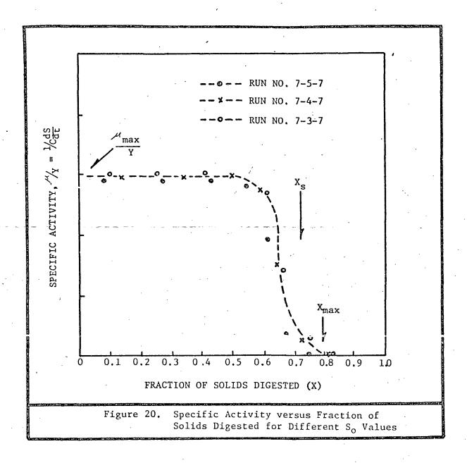
fraction of substrate degraded in the standard substrate test (from Figure 5) is about 0.72. The range of  $X_{\rm max}$  values obtained in the three fermenters was from 0.75 to 0.82 which compares favorably with the predicted value obtained in the shake-flask test.
