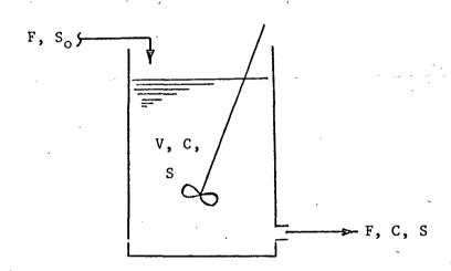
Using the system and culture growth parameters, a general material balance may be written around the fermenter for cells and for substrate.
