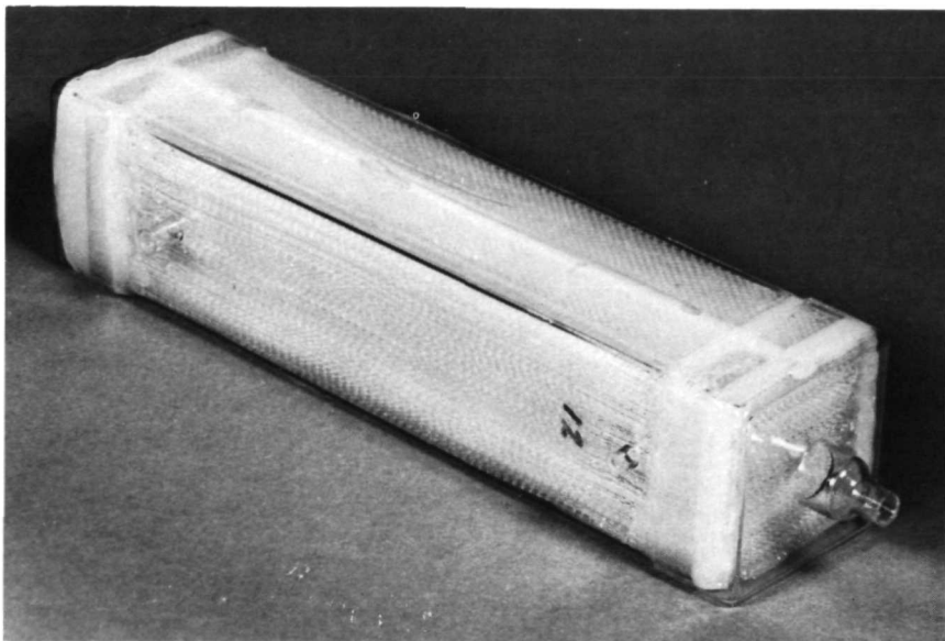
FIGURE I.17 Preliminary version of a small, inexpensive artificial kidney, which has been developed at the High Energy Facilities Division of Argonne National Laboratory.
