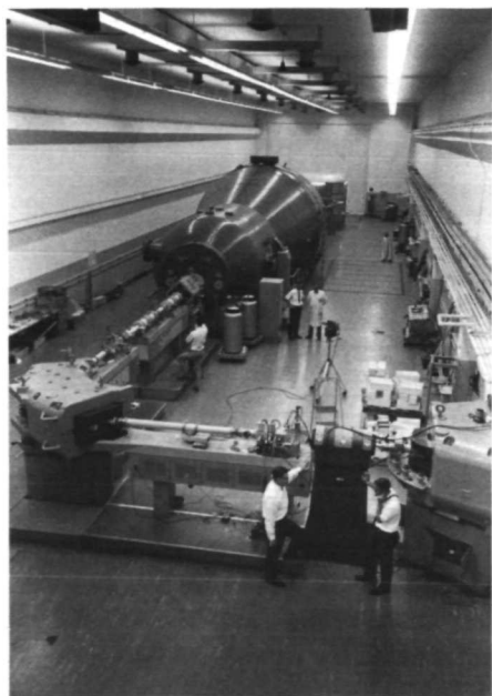
FIGURE II.6 The first of the Emperor class of electrostatic Van de Graaff accelerators, installed in the Arthur Williams Wright Nuclear Structure Laboratory at Yale University. This accelerator is the largest of the tandem configurations in research use and is the first to make available all the nuclear species to precision study. Terminal potentials in excess of 11 MeV have been obtained on the machine.
