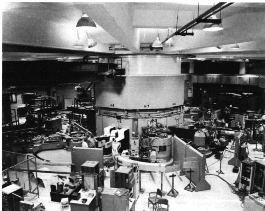
FIGURE II.8 The Brookhaven High Flux Beam Research Reactor. This heavy water, 40-MW reactor has been in operation since 1965. The thermal neutron flux is 7 \times 10^{14} (n/cm 2 /sec).
