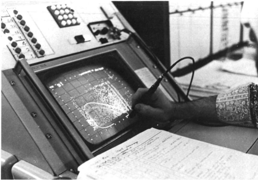
FIGURE II.16 View of the oscilloscope display of the on-line computer used with the Maryland cyclotron. The display illustrates typical nuclear data accumulated during experiments and the interaction of the computer through a light-pen.
