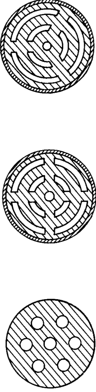
Figure 25.—Typical multiperforated grain shapes.
