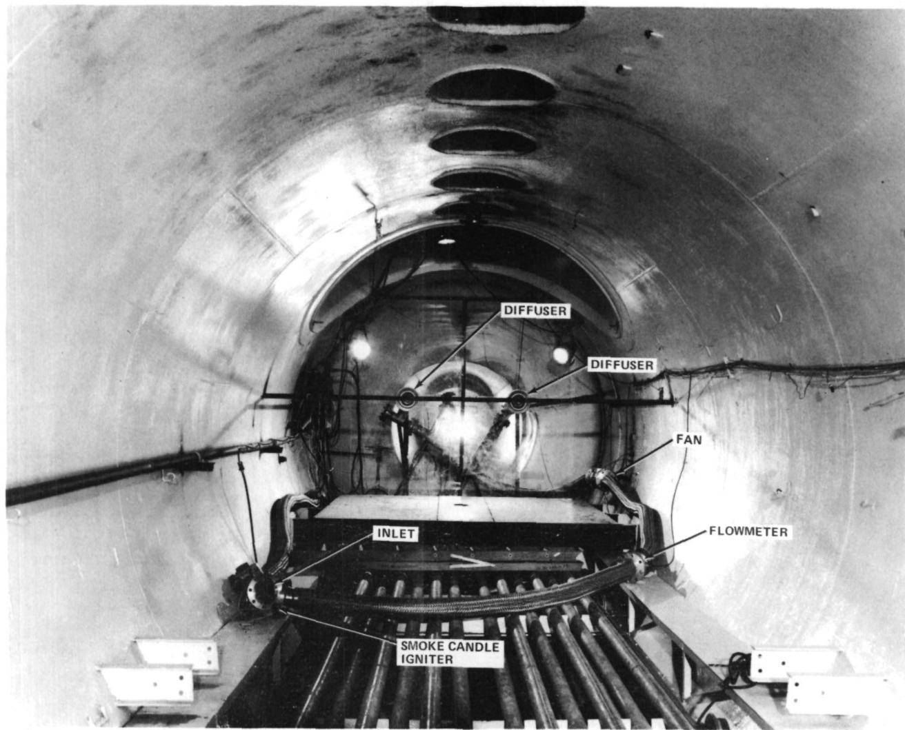
Figure 22. Diffuser test setup in vacuum chamber.
