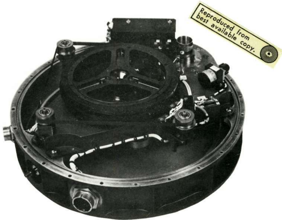
Figure 2-V-98. SR Tape Transport Top View, Dome Removed
