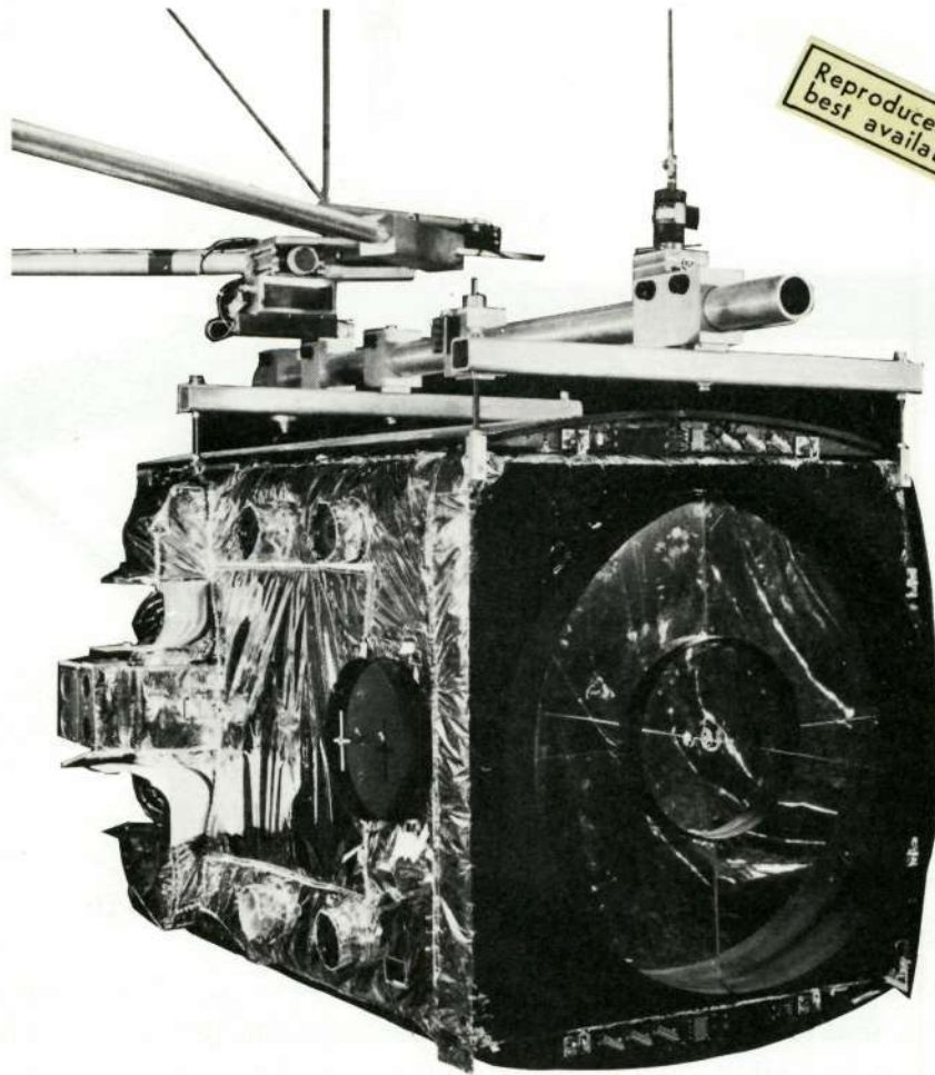
Figure 3-V-7. ETM Spacecraft Suspended from Bifilar Pendulum
