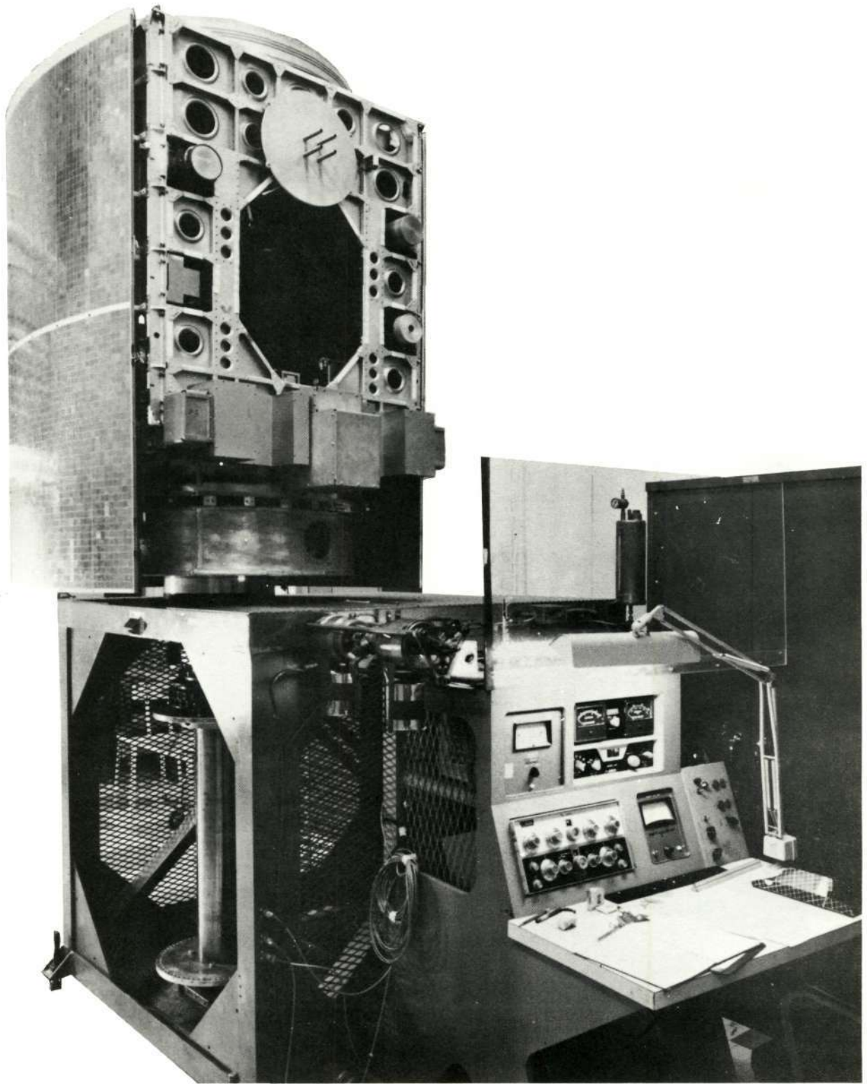
Figure 3-II-2. MTM on Dynamic Balance Machine
