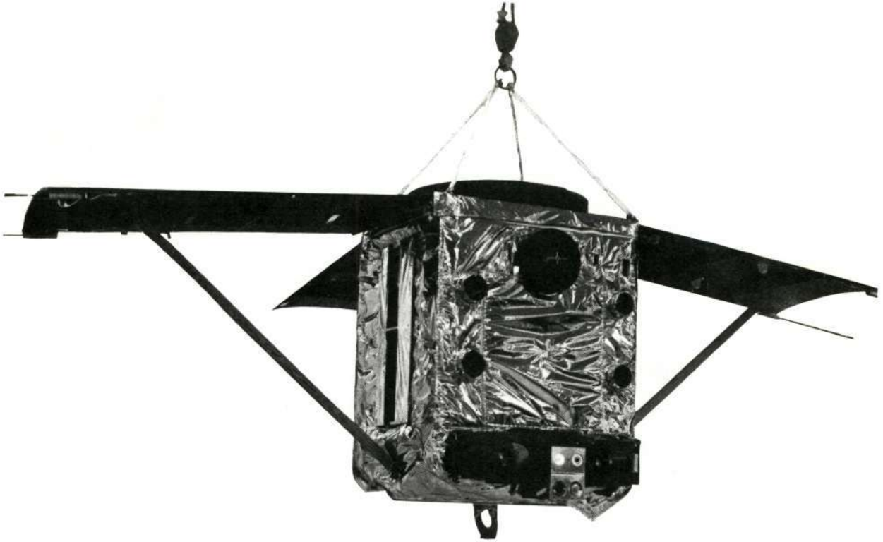
Figure 3-V-6. RFI Test of ETM Spacecraft
