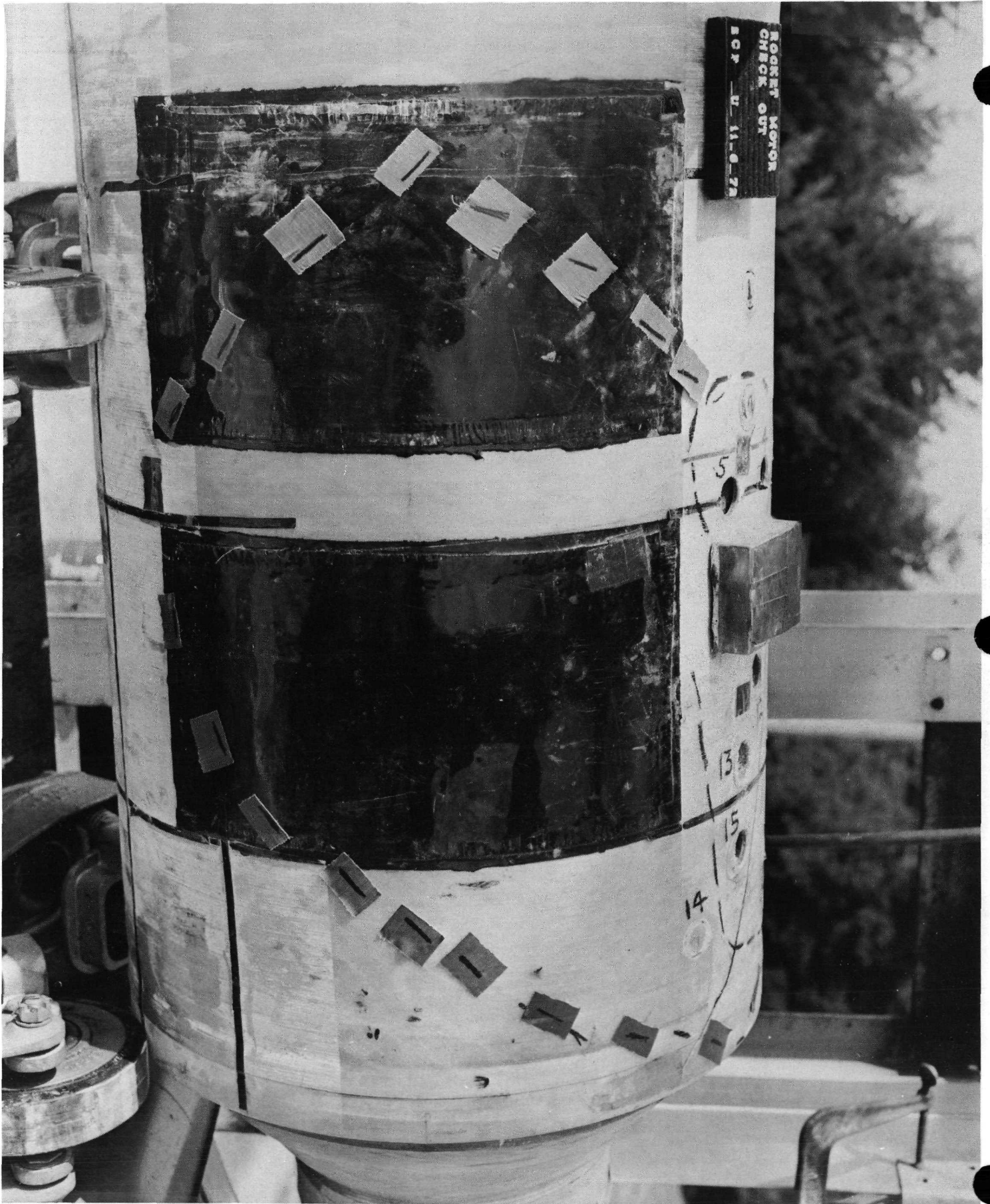
Fig. 77 Trace of Separated Area Between Liner and Propellant Detected by Feeler Gage During Destructive Tests on Motor S/N 424
