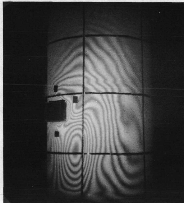
Fig. 53 Interference Field of Hologram No. 131 Which Occurred After Cyclic Heating Test 3T
