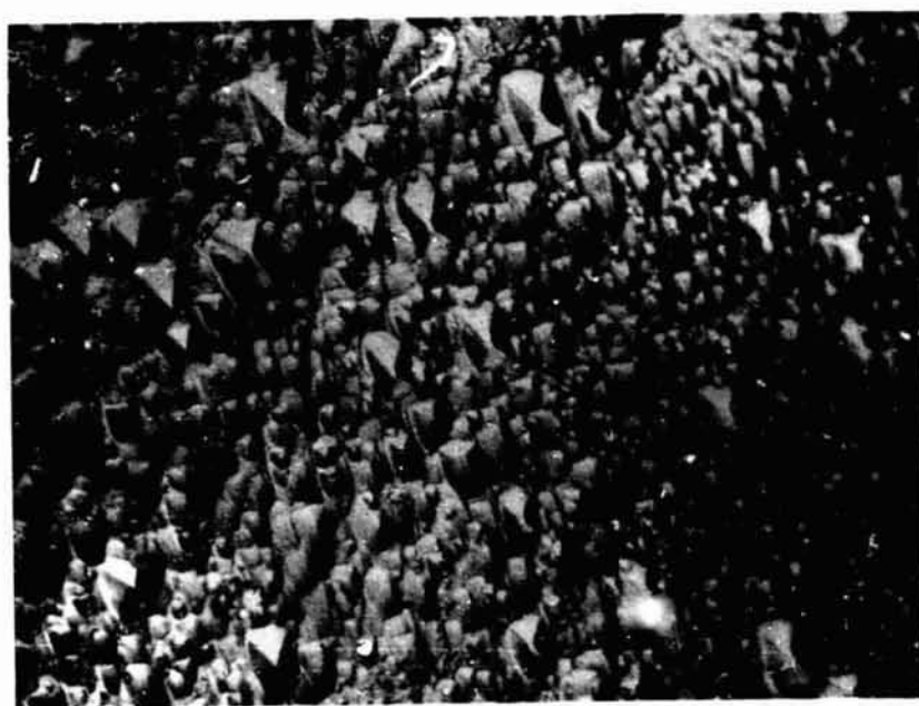
Fig. 5. Etch pits on (100), Richardson-Crocker etch, dislocation density 4 \cdot 10^5/\text{cm}^2 .
