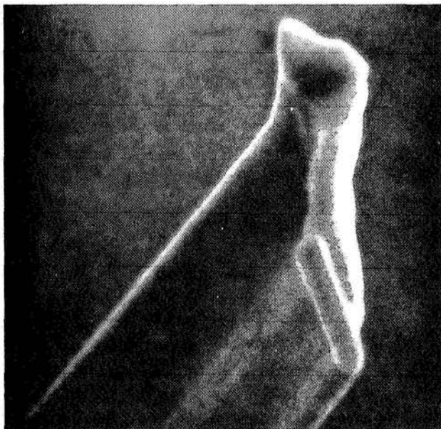
Fig. 1 A scanning electron microscope photograph of the tip of an InBi whisker. The bend at the tip is the result of an attempt to cleave the whisker. Note "celery stick" appearance which reveals no indication of crystal symmetry.
