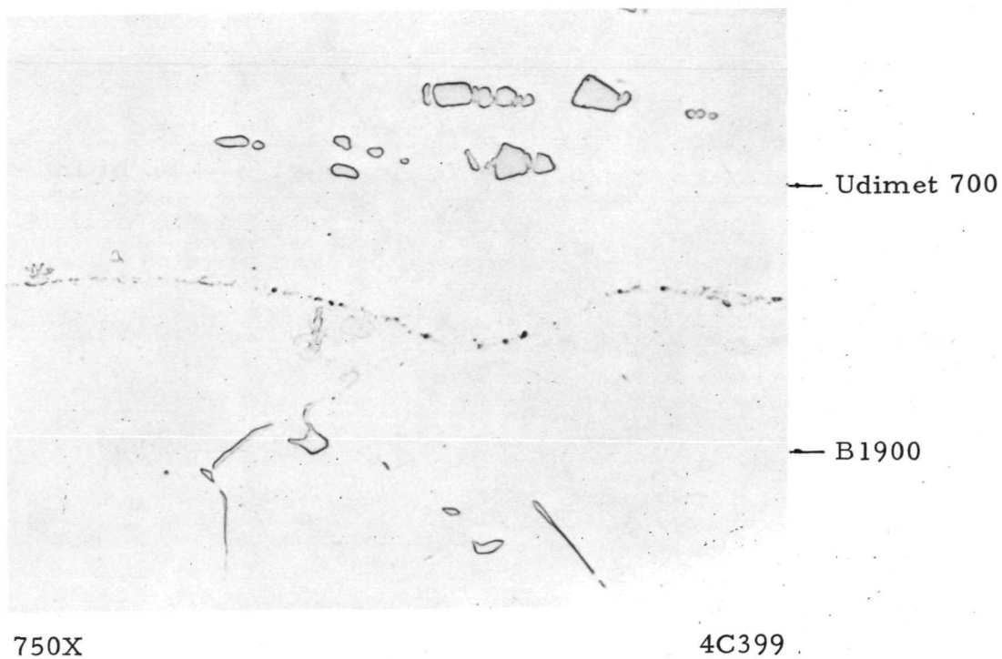
c. As-Polished View at Higher Magnification
