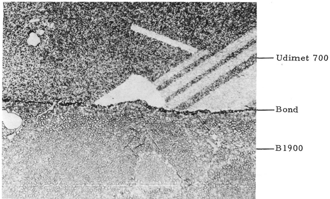
b. Higher Magnification View of Electroetched Surfaces
