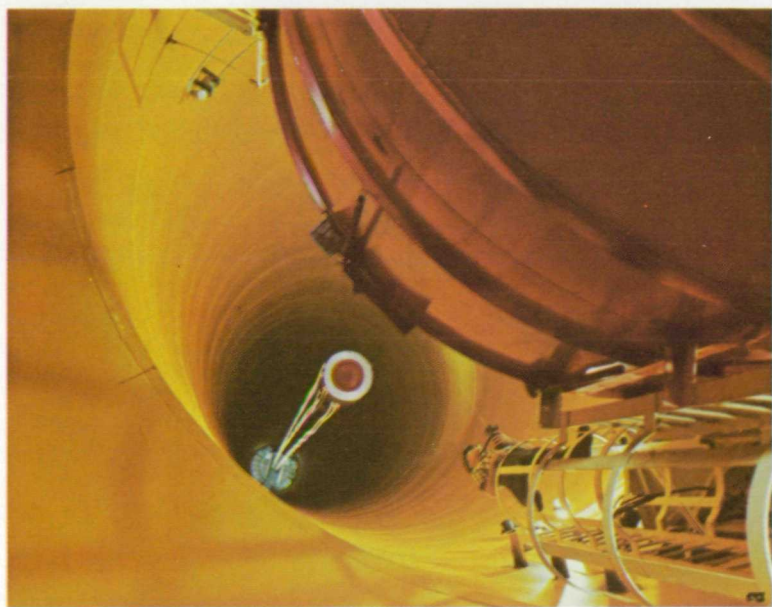
A photograph of the Zero Gravity Drop Tower at Lewis Research Center in which photographic equipment is in the drop packages to record test events.
