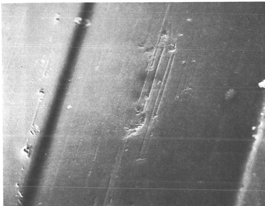
Fig. C.5-34 — Scanning electron microscope photograph of surface defects of master grating occlusions replicated in prismatic grating (1,660 \times )
