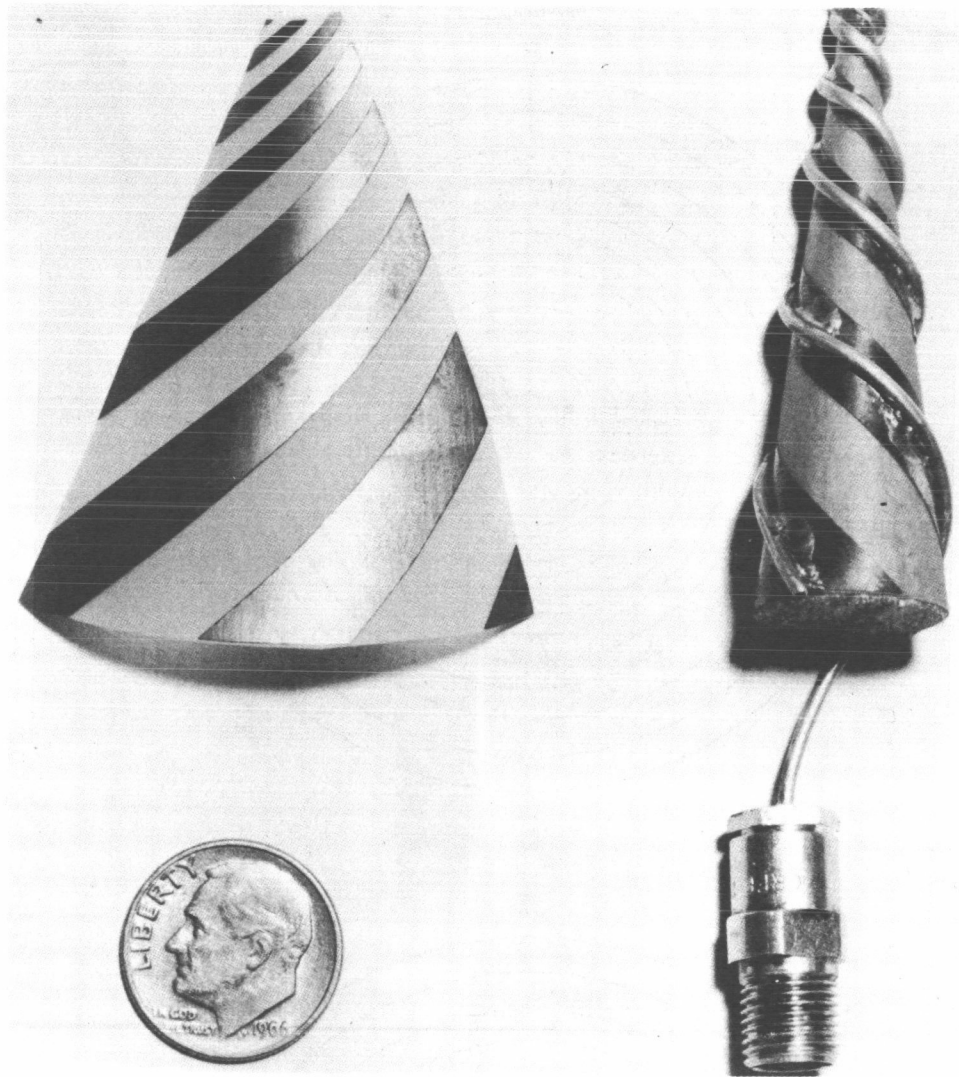
Figure V-7. One-fifth scale model conical spiral antenna frequency — 11.0 GHz.
