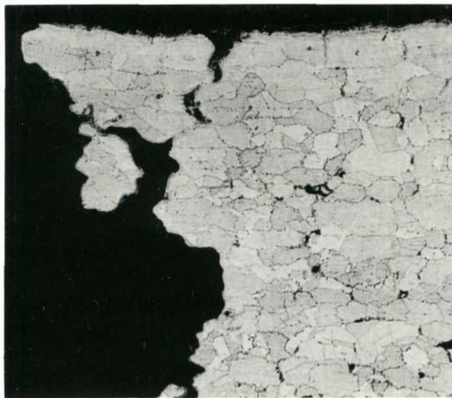
a) 17.7 hours rupture life, 100X ASTM grain size No. 6.
