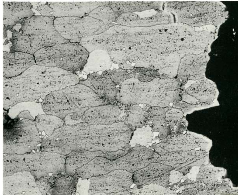
b) Base + VC (0.28 w/o C), 47.9 hours life, ASTM grain size No. 2-4.
