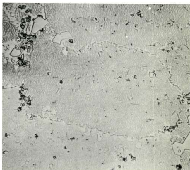
d) Base alloy + VC (0.28 w/o C) side press + 24 hours at 2400°F (1315°C) vacuum + 1975°F (1090°C) A + 24 hours at 1700°F (927°C) air cool, 500X, etched.
