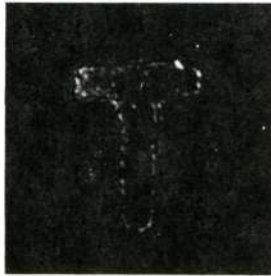
Figure 11a. Impulse Response of a Gradient Correlation Filter for the Letter T Synthesized by a Multiple Exposure Technique
