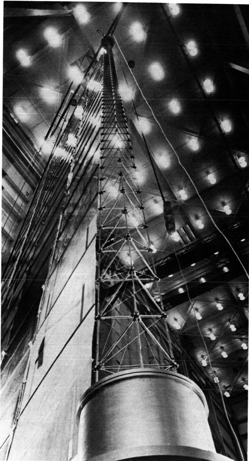
Figure 7. - Extendible truss beam.
