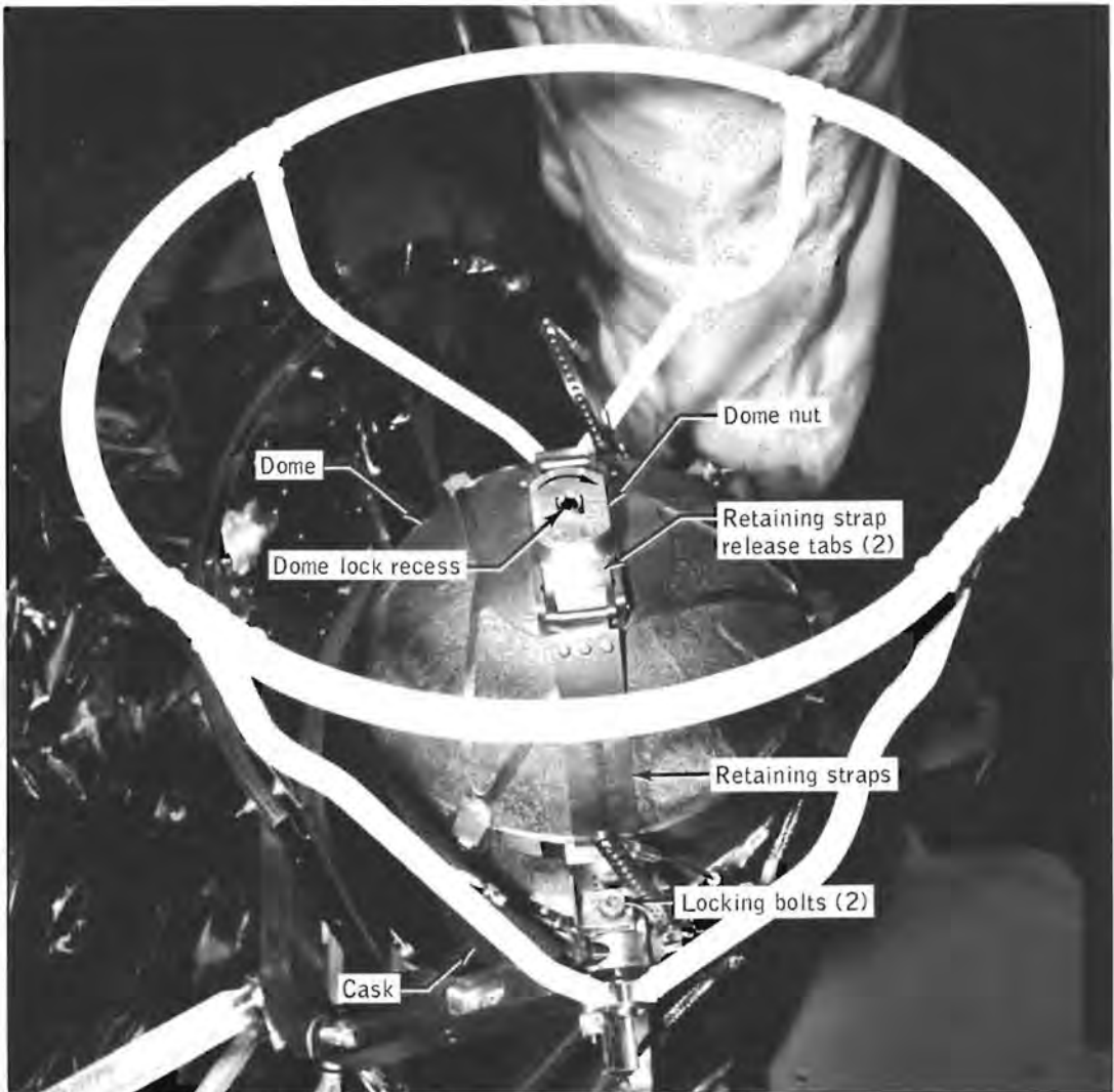
Figure 15-22.- Fuel cask dome release mechanism.
