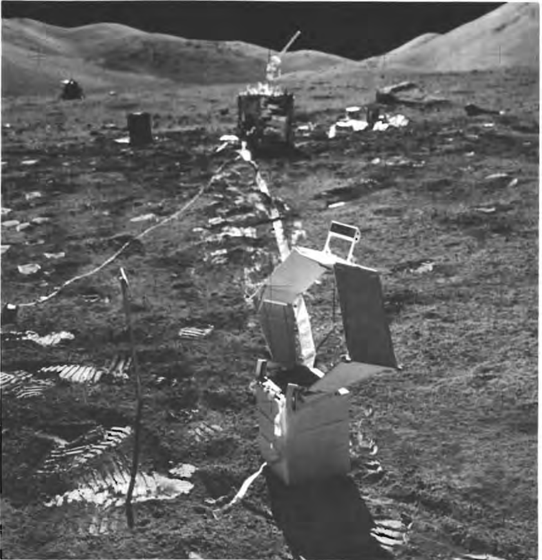
Figure 10-7.- Lunar surface gravimeter.
