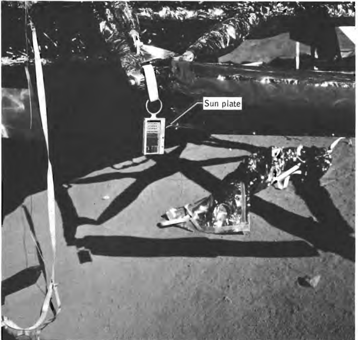
Figure 10-13.- Cosmic ray experiment showing sun plate.
