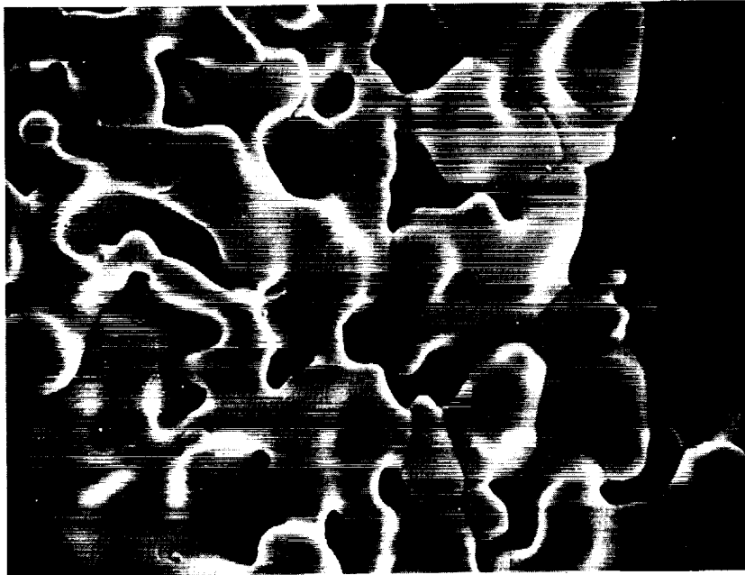
Figure 3-2 TUNGSTEN FOAM SURFACE ROUGHENED BY DEPOSITION OF ADDITIONAL TUNGSTEN POWDER, 3000X
