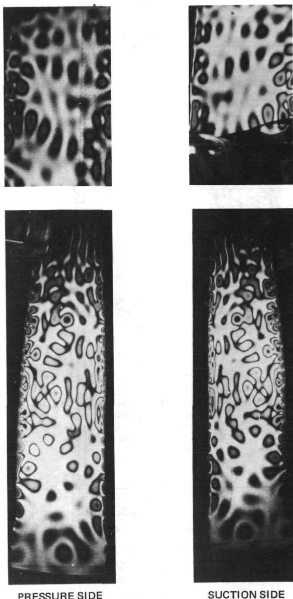
Figure 6.—Holographic reconstructions of a good airfoil. Note the exact correspondence of the mode patterns over the entire surface of both sides, verifying that it is vibrating as a structural entity.
