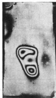
Figure 8.—HNDT with pressure stressing as applied to a resistance-welded rigid metallic structure (a, deicing vane) and an adhesively bonded compliant material (b, rubber plies). The former illustrates the use of the moiré technique to desensitize holographic interferometry so that the fringe shape is more clearly apparent, while flaw detection sensitivity is maintained. The latter illustrates the use of both the pressure relaxation and pressure differential methods.
