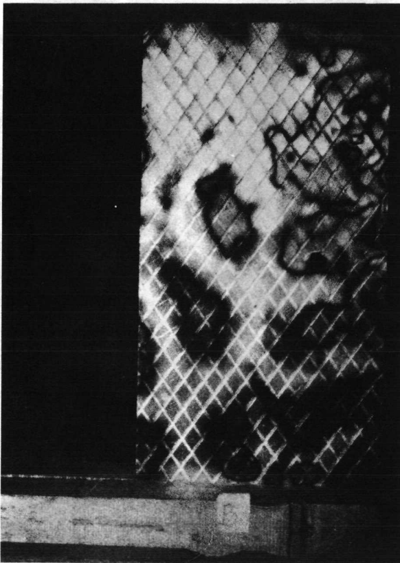
Figure 11.—Disbond detection in electron-beam-welded honeycomb sample.
