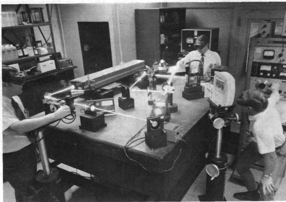
Figure 18.—Real-time vibration analysis system in operation.
