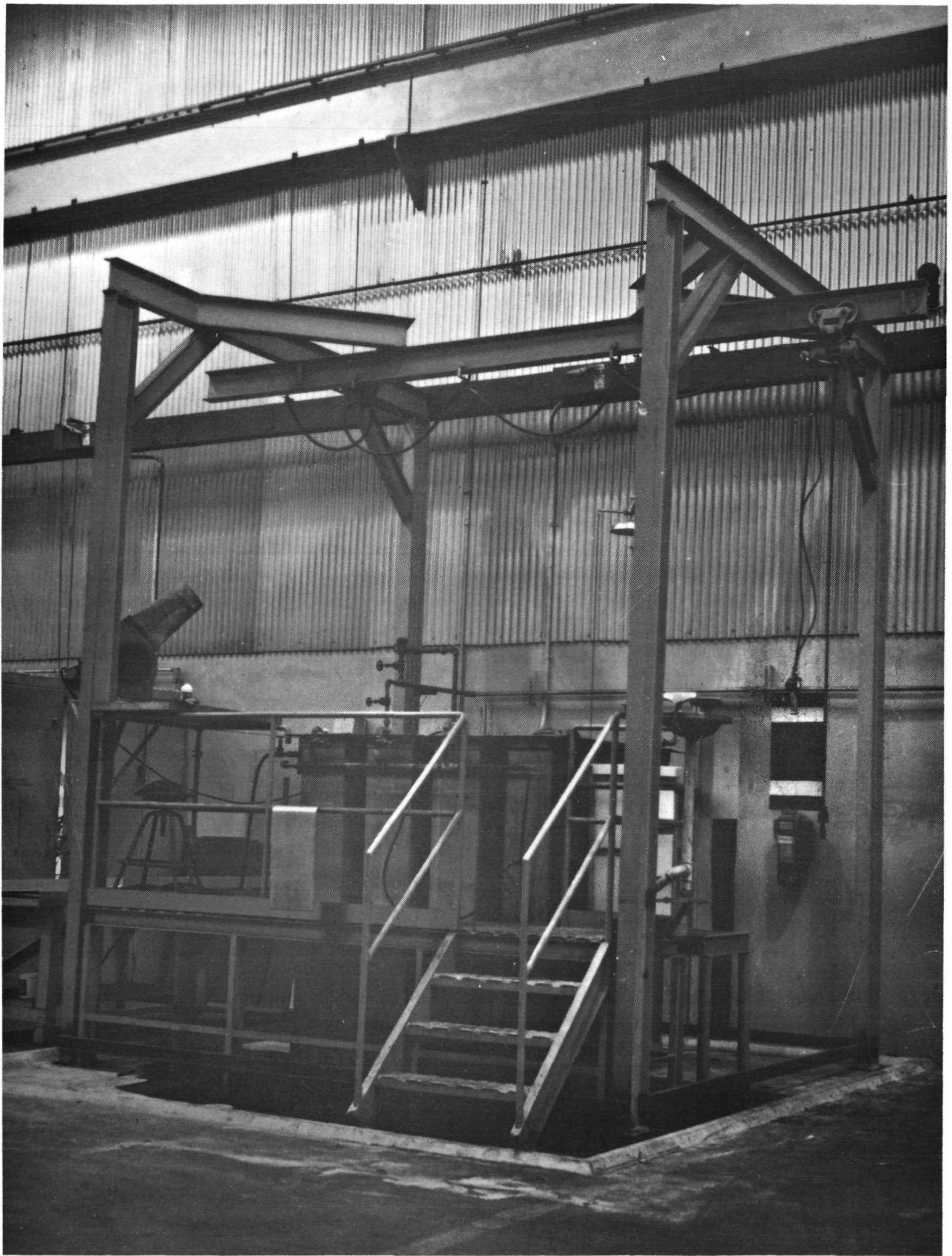
FIGURE 1. ALUMINUM FOIL AND BORON FILAMENT CHEMICAL CLEANING TANKS
