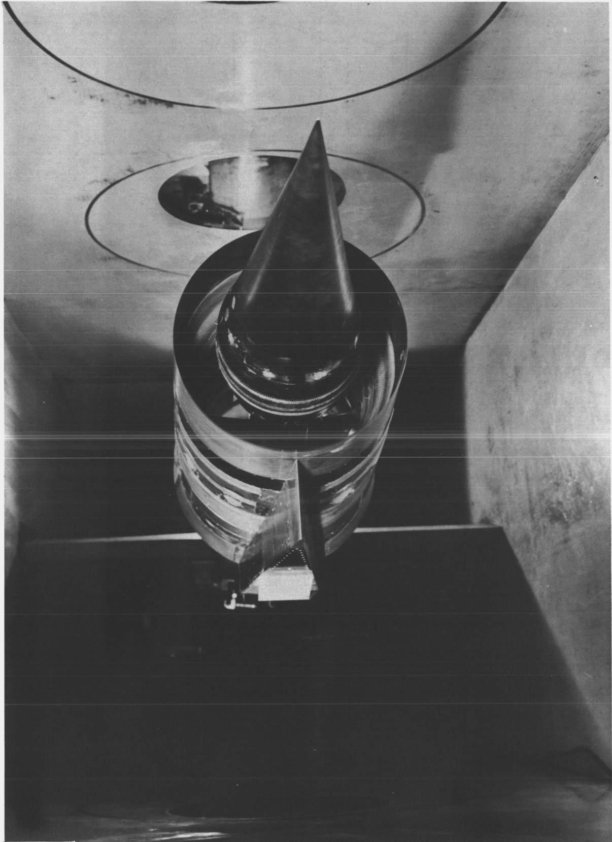
Figure 1.- Model mounted in the wind tunnel.
